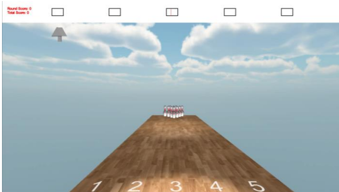
Fig. 3: The mVEP HUD within the bowling game. The arrow detailing what stimulus the player should be concentrating on is below the first stimuli. The 3 rd stimuli is currently active with the red bar being approximately mid-animation.
