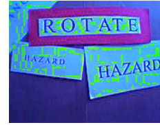
Figure 8. Camera distortion due to lighting conditions
