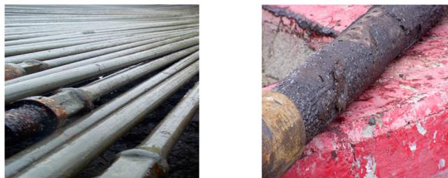
**Figure 2.** Pictures of sucker rods without and with paraffin deposition from positive (left) and negative (right) wells, respectively. Obviously the effectiveness of a microbial treatment of prevention wax from precipitation is easily measured by detecting paraffin in the surface of sucker-rods.
