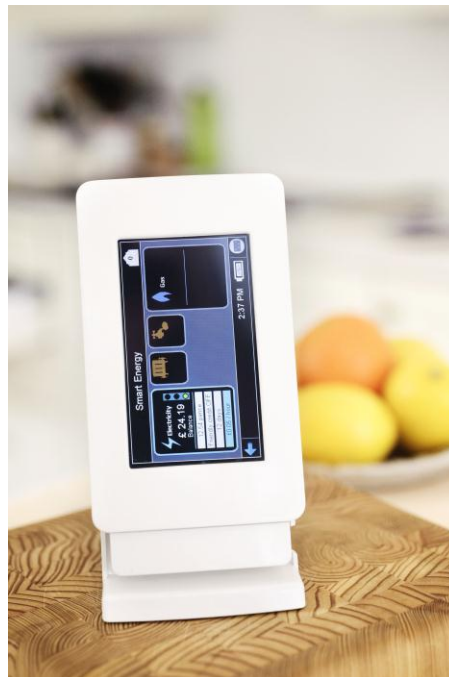
Figure 3.7. The SMART meter’s in-house display
