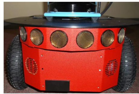
Figure 2. The real-life positioning of the ultrasonic sensors in the array. Sensors S1-S6 are clearly visible as the forward facing sensors on the Pioneer 3DX; sensors S0 and S7 are positioned to the left and right of the array respectively.
