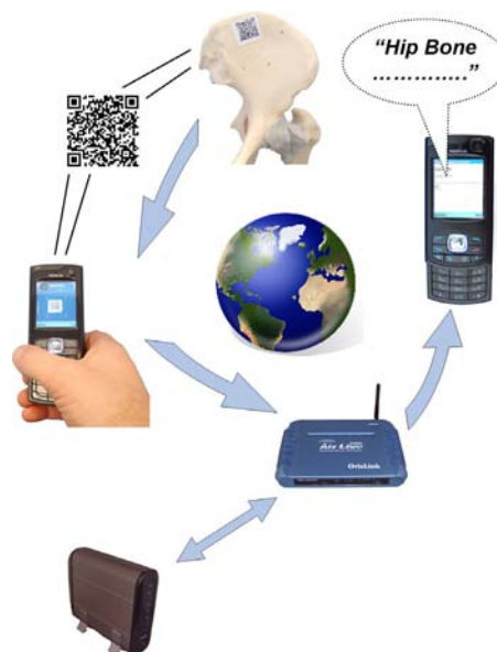
Figure 1. Illustrating the process of using 2D barcodes attached to objects, linked to audio files.
