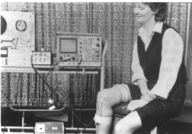
Fig. 1 Early investigations of knee vibration were carried out using a miniature accelerometer taped over the patella and an oscilloscope to view the vibration waveforms
