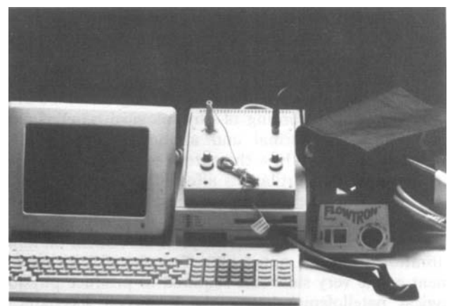
Fig. 8 A system devised for early detection of deep vein thrombosis consisted of a computer, small pump, thigh cuff and strain gauge
