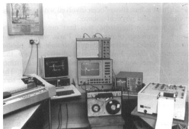
Fig. 2 A system was devised to analyse any human joint vibration consisting of reel-to-reel tape, spectrum analyser, oscilloscope, Apple computer and hard-copy devices
