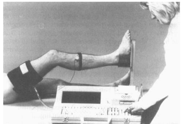
Fig. 9 The preproduction prototype of the 'clot-spotter'—a screener for deep vein thrombosis—shown attached to a subject undergoing examination
