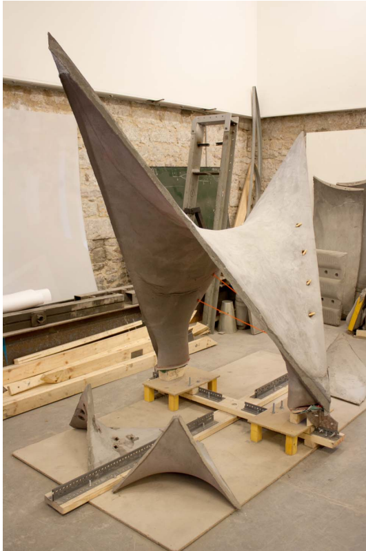
Figure 13. Edinburgh's curved shell experiments
