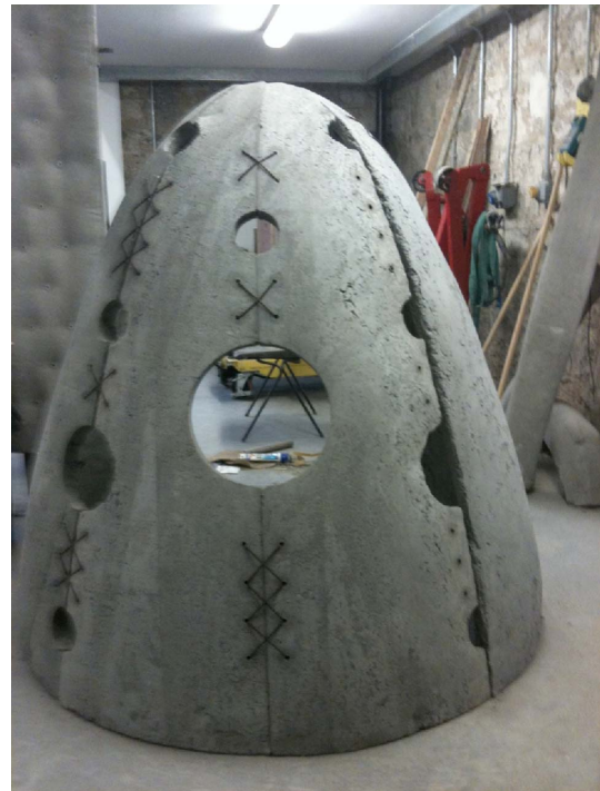
Figure 4. Curved formwork shell structure
