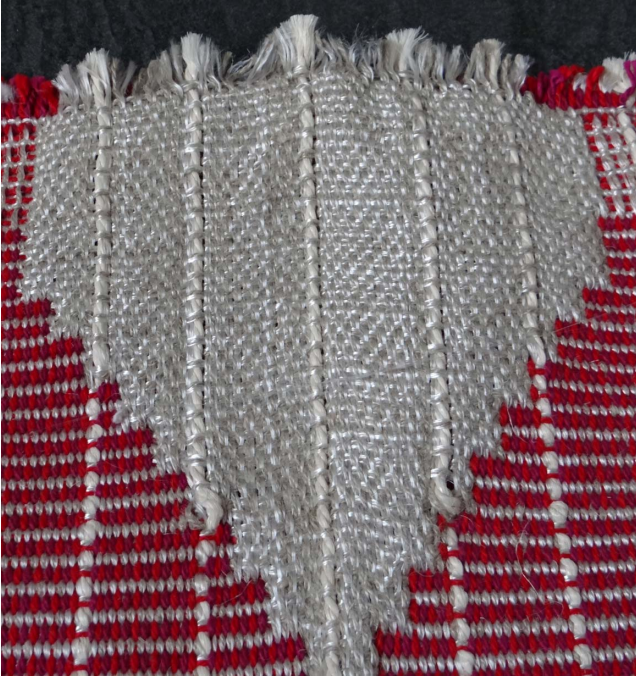
Figure 11. Tapered 3D woven preform
