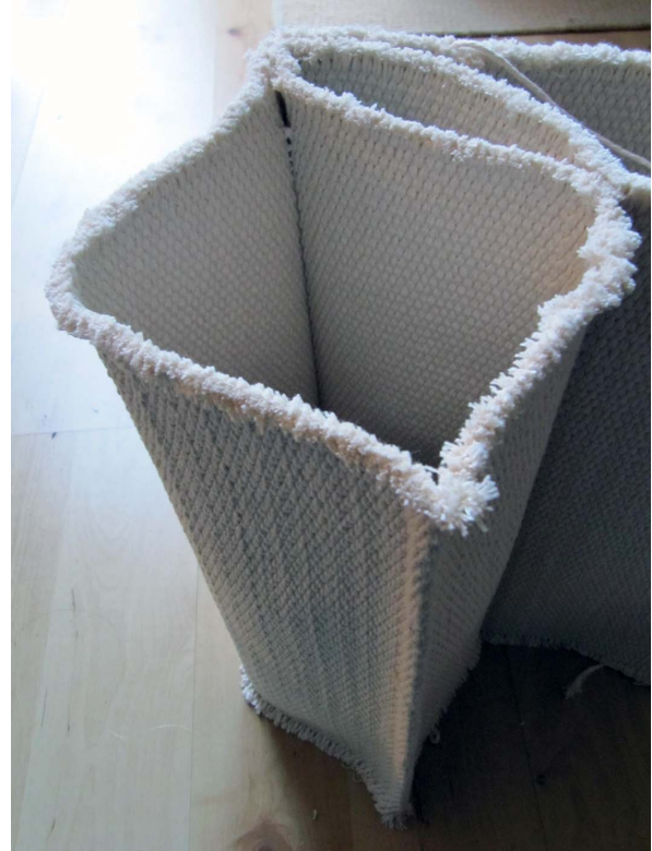
Figure 10. Three-dimensional woven material
