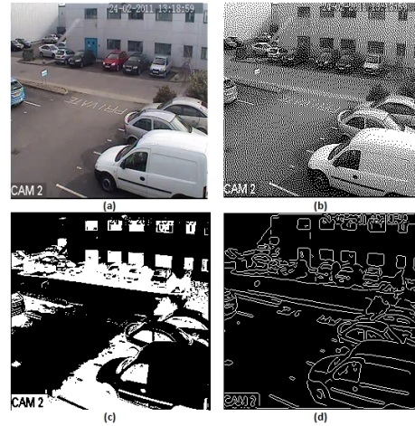
Fig. 2. (a) original image. (b) created by dithering using the method described by Floyd and Steinberg [7], (c) created by thresholding the original image and (d) created by Canny edge operator respectively.
