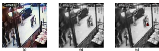
Fig. 8. (a) found image from the Web. (b) extracted hidden content and reconstructed using WinHD. (c) altered region is shown with red color.
