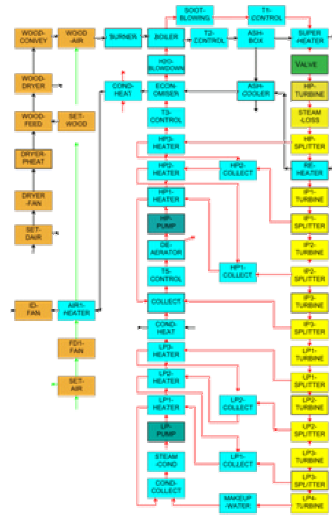
Figure 3: PFD of 'Port Talbot type' CFBC
