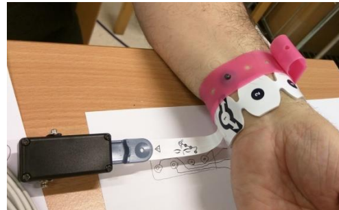
Figure 3. BIS-Quatro sensor strap with fixing dry electrodes elastic band on the wrist.
