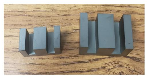
Fig. 3. Examples of Ferroxcube EE type cores. [Image by author]
