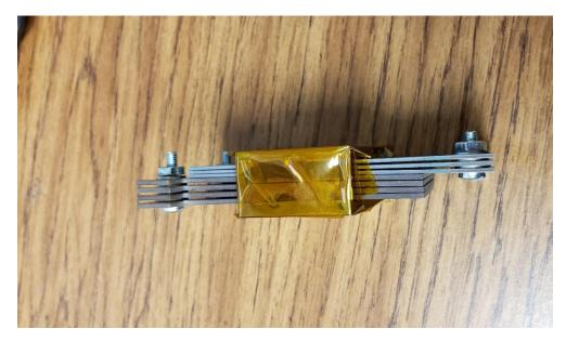
Fig. 13. Assembled planar transformer – side view. [Image by author]
