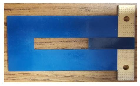
• 5 PCB (15.5A per winding layers) – trace width = 18.1 mm
