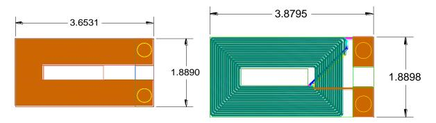
Fig. 16. (a) Primary LTCC board dimension (b) Secondary LTCC board dimension. [Image by author]
