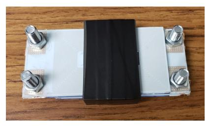
Fig. 25 Assembly of LTCC transformer. [Image by author]
