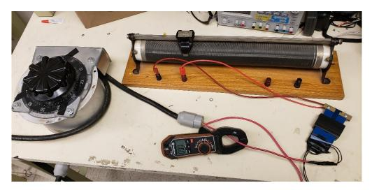
Fig. 15. OC testing arrangement for the planar transformer. [Image by author]
