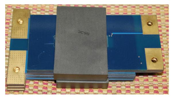
Fig. 7. Example of core mounting and assembling the planar transformer. [Image by author]
