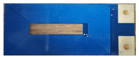
Fig. 9 (a). Secondary winding in PCB- top layer. [Image by author]
