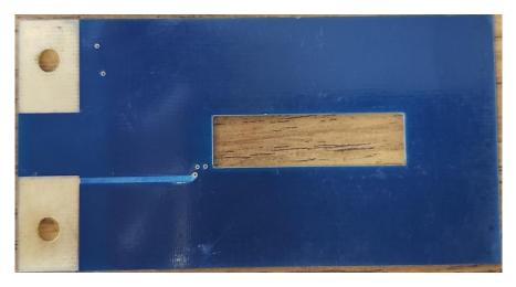
Fig. 9 (b). Secondary winding in PCB- bottom layer. [Image by author]
