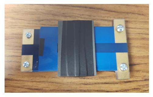
Fig. 12. Assembled planar transformer- top view. [Image by author]
