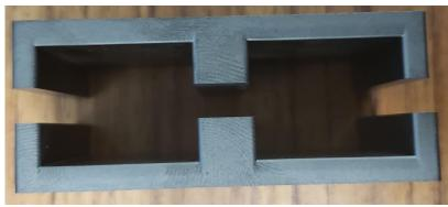
Fig. 11. Planar transformer core- perspective. [Image by author]
