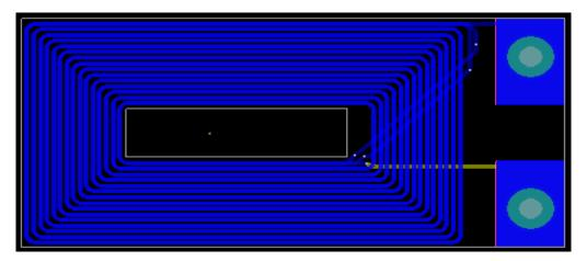
Fig. 6. PCB windings- low current trace. [Image by author]
