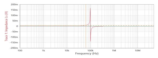
Fig. 27 Inductance vs frequency plot from the bode analyzer. [Image by author]
