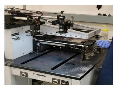
Fig. 23. Thick film screen printer for LTCC printing technology. [Image by author]
