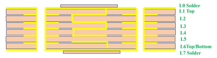
Fig. 18 2D design of secondary LTCC board. [Image by author]
