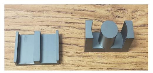
Fig. 4. Examples of Ferroxcube EI an ER type core. [Image by author]
