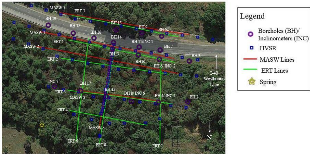
Figure 7- Testing Locations for Borings and Geophysics for Ozark (Retrieved from Google Earth)
