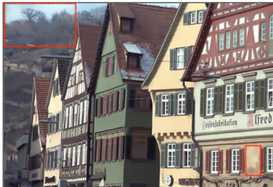
Figure 4.8: Picture compressed with BPG (RGB 4:4:4), QP = 42, compression level = 9, bpp = 0.835. Red box areas look blurred.
