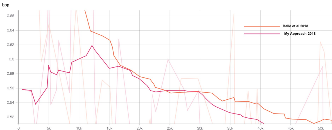
Figure 4.12: Comparison of bpp (bits per pixel) in the first 50K training iterations between Ballé’s approach in 2018 and our 2018 approach.
