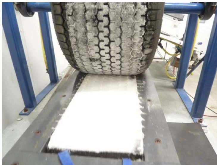
Figure 1. Trafficking machine in action in the MSU Subzero Lab.
