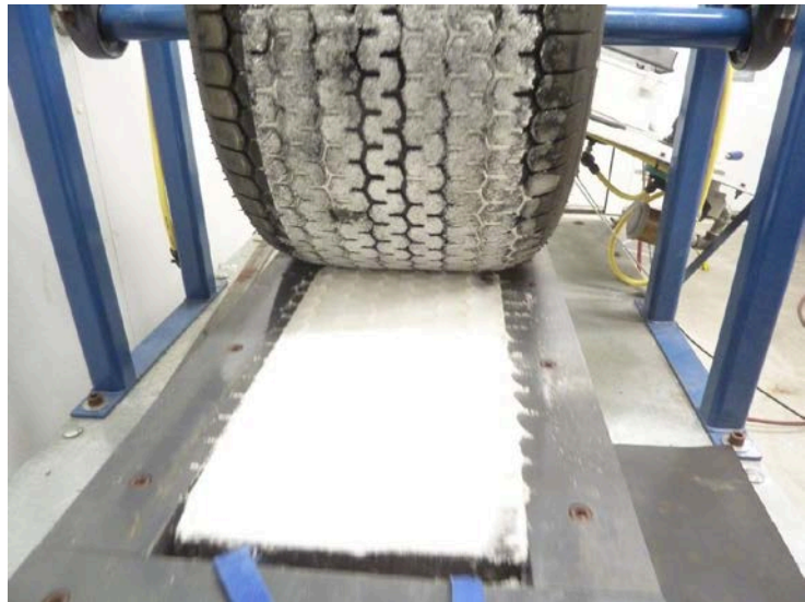
Figure 2. Custom trafficking device in the MSU Subzero Lab environmental chamber, trafficking an asphalt sample with snow.
