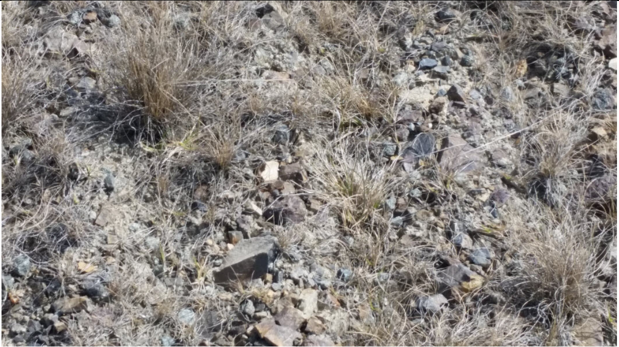
Figure 1.1 Dalton, MP 11–18 reconstruction, bid Jan. 2012, 1% for seeding. Tracked side slope, dead grass in tracks. Sparse grass in clumps.
