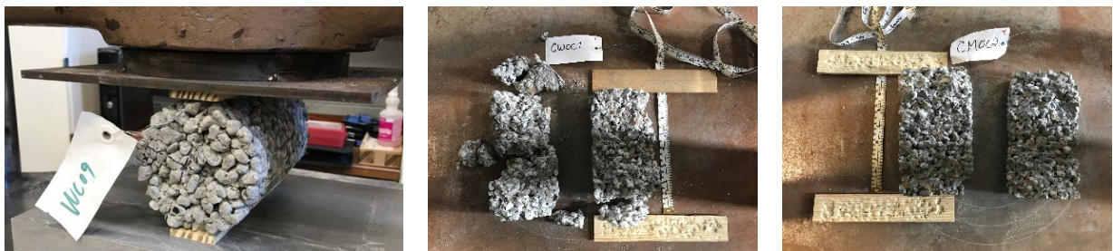
Figure 2.5 Split tensile test procedure (left) and broken specimen examples
