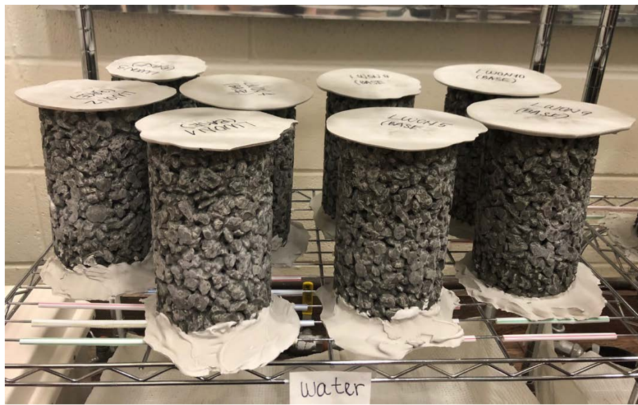
Figure 3.8 Capped specimens before unconfined compressive strength test: Phase IIb
