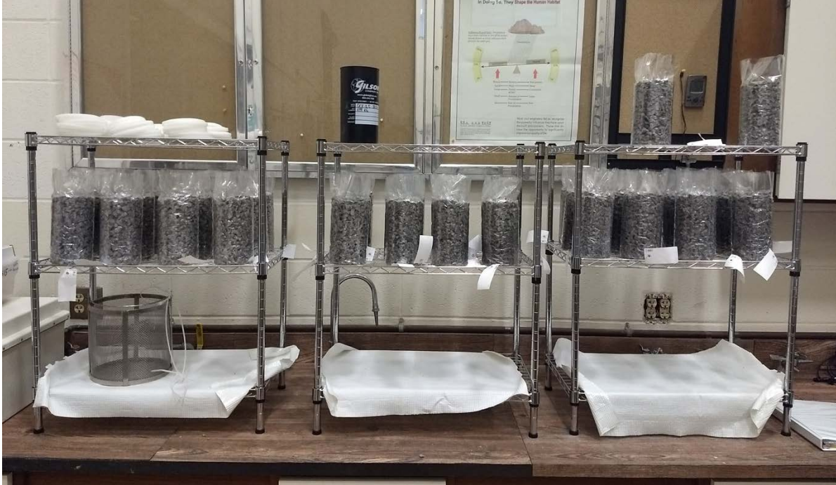
Figure A.2 Specimens on the drying racks with the absorbent pads below
