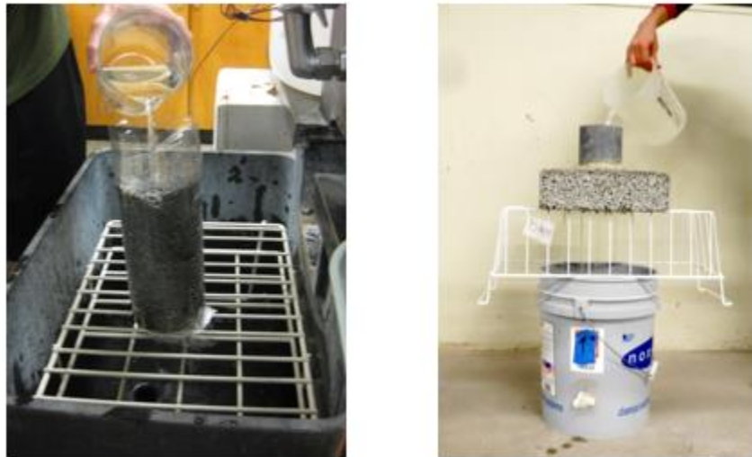
Figure 2.4 Infiltration test performed on 4-inch PC cylinder (left) and on PC slab (right)
