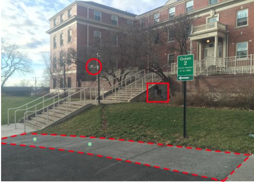
Figure 2.10 Project boundary showing location of sensor trees (green dots on the sidewalk), solar sensor (red circle) and datalogger (red box) with respect to the PC sidewalk (red dashed line).
