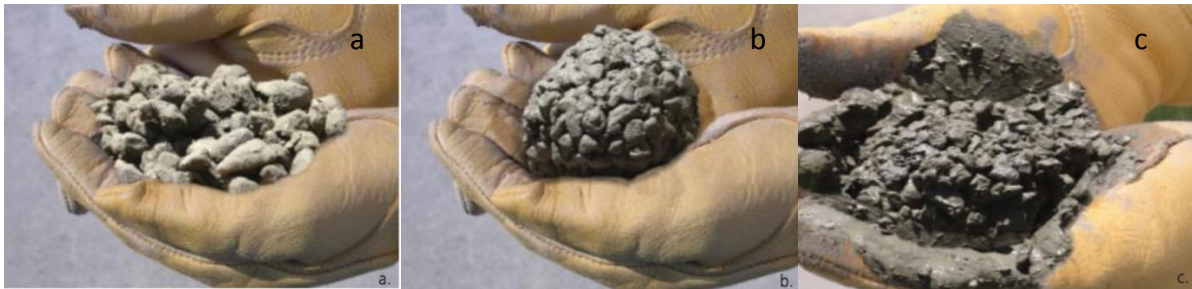
Figure 2.7 Samples of pervious concrete with different water contents, formed into a ball: (a) too little water, (b) proper amount of water, and (c) too much water (reprinted from Tennis et al. 2004)
