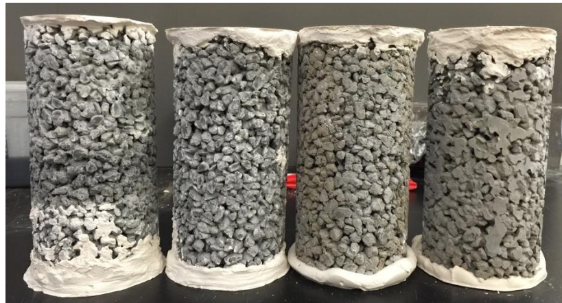
Figure 4.1 Pervious concrete cylinders with capping: (left to right) cement, cement + GO, fly ash, fly ash + GO
