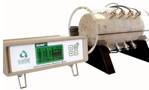
Figure 3.3 Surface resistivity test setup (reprinted from GIATEC)
