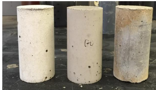
Figure 3.22 Mortar cylinders, 2 inch \times 4 inch in size: cement mortar (left); GO-modified fly ash mortar (middle); fly ash mortar (right)
