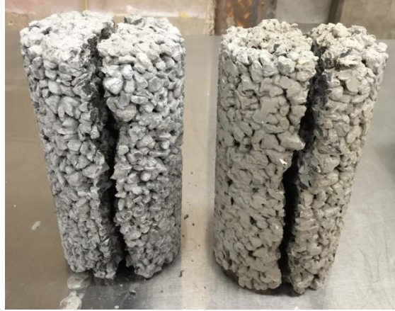
Figure 4.9 Failure surface of samples after split tensile strength tests at 7-day: cement + GO(left); fly ash + GO(right)
