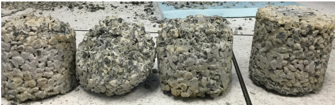
Figure 4.19 Pervious concrete samples after the third cycle during freeze-deicer salt scaling test (top to bottom) cement, cement + GO, fly ash, fly ash + GO
