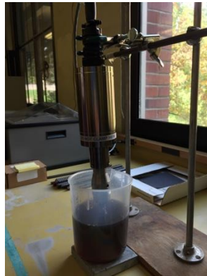
Figure 3.21 Ultrasonification of GO suspension
