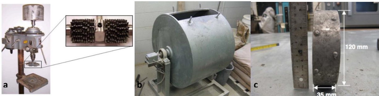
Figure 2.14 Abrasion testing apparatus (a) ASTM C944 method; (b) L.A. abrasion machine; (c) studded steel wheel abrasion test (reprinted from Dong et al. 2013)
