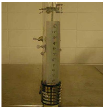
Figure 2.10 Permeameter used to measure the permeability of pervious concrete samples (reprinted from Das and Sobhan 2013)
