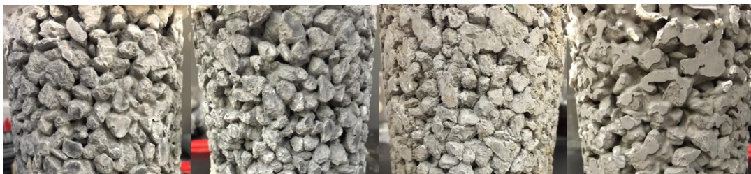
Figure 4.2 Close-up view of sample surface: (left to right) cement, cement + GO, fly ash, fly ash + GO
