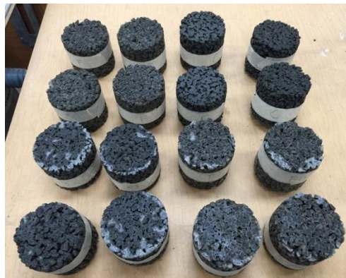
Figure 4.16 Pervious concrete samples before freeze-deicer salt scaling test
