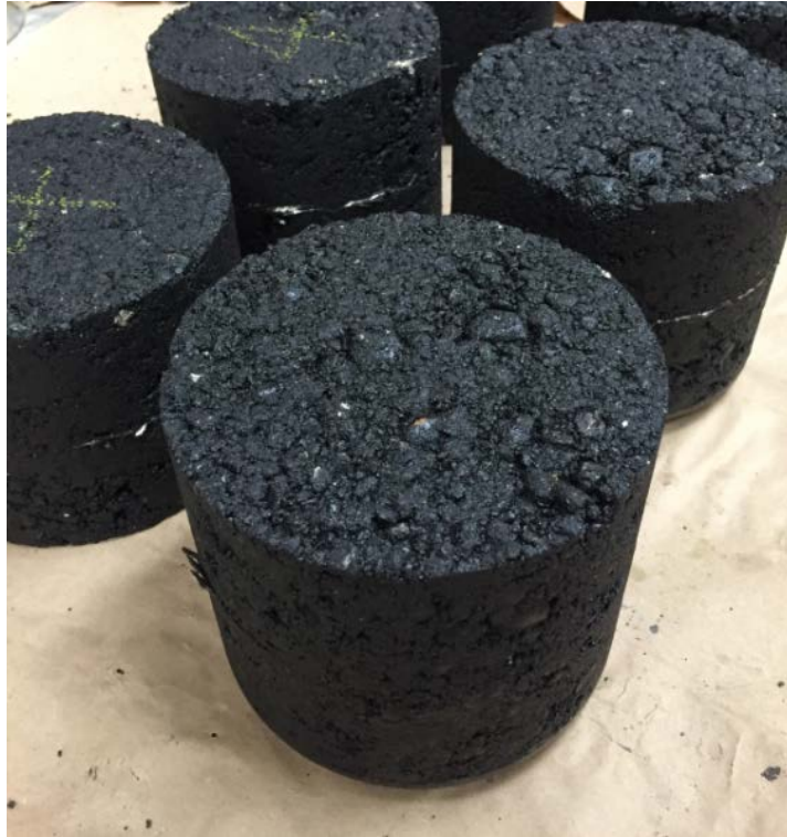
(d) Specimens compacted for the overlay, IDT tests, and dynamic modulus test in IDT mode
