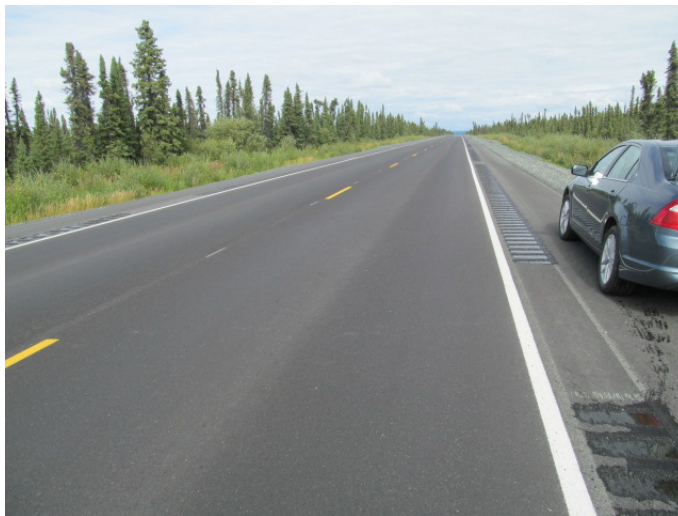
Figure 3.21 G50/50 test section (reinforced with 300 feet of G50/50 in the left lane in area 9, no visible cracks)
