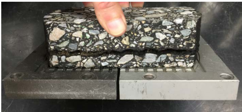
Figure 2.8 Specimen debonding during overlay testing
