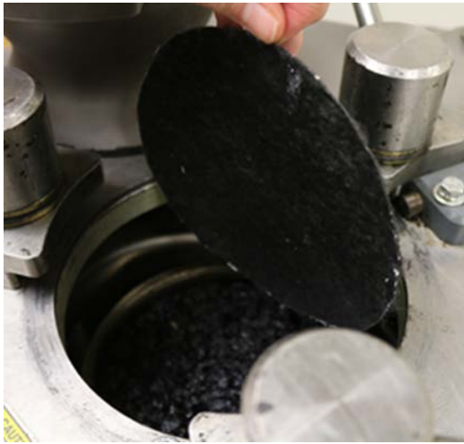
(c) Bottom layer of the specimen (entire interlayer or interlayer strip)
