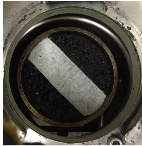
(c) Bottom layer of the specimen (entire interlayer or interlayer strip)
