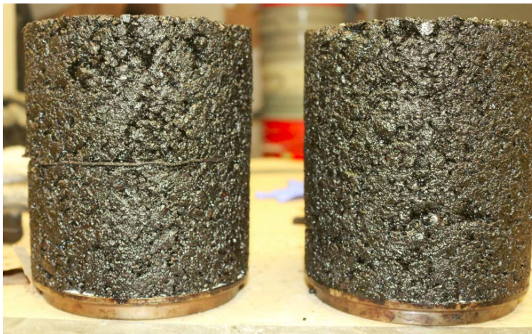
(e) Specimens compacted for the dynamic modulus test by the AMPT (patching group at left, control group at right)
