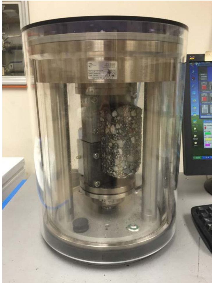
Figure 2.6 Overlay test setup
