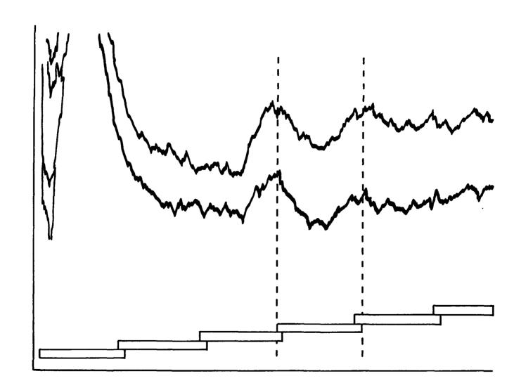
Fig. 11. Vertical lines are dropped from the 2 peaks to the calibration marks below (30 and 41 msec respectively). The difference between these 2 intercepts, <u>i</u>. <u>e</u>. 11 msec., is divided into the measured distance between the 2 electrodes on the finger (4.3 cm) giving a conduction velocity of 39.0 m/sec
