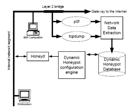
Figure 12, Dynamic passive scanning honeypot implementation [Hieb & Graham, 2004]
