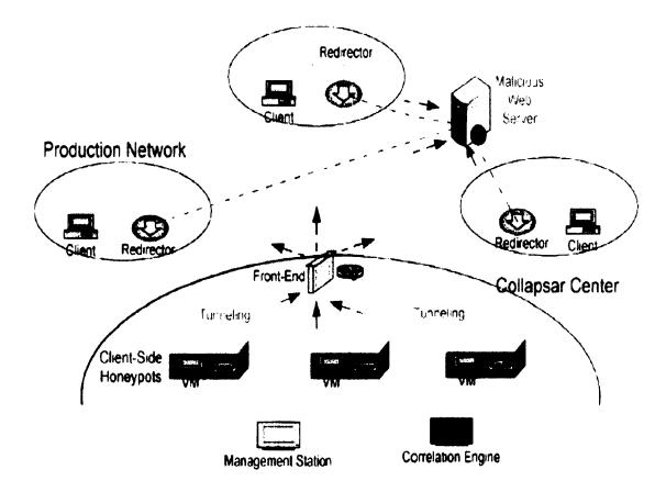
Figure 8, Collapsar reverse honeyfarm architecture [Jiang et al., 2006]
