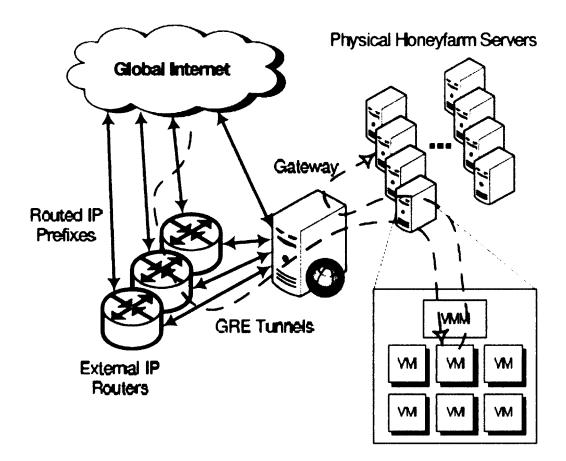
Figure 9, Potemkin virtual honeyfarm architecture [Vrable et al., 2005]
