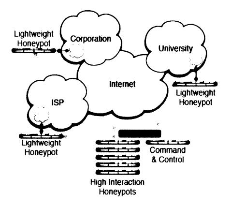
Figure 6, Hybrid honeypot architecture [Bailey et al., 2004]
