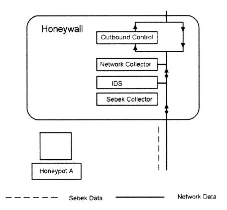
Figure 4, Honeywall Diagram [Balas & Viecco, 2005]
