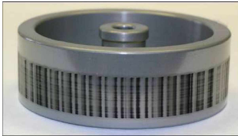
Figure 2.6. An example drum with collected aerosol. This drum (not from this study) has been used to collect aerosol over an extended period. The dark lines are likely heavy industrial pollutants and carbon soot. The lines on the drum surface result from the internal slotted orifice directing aerosols to impact on the drum surface over a discrete time interval.
