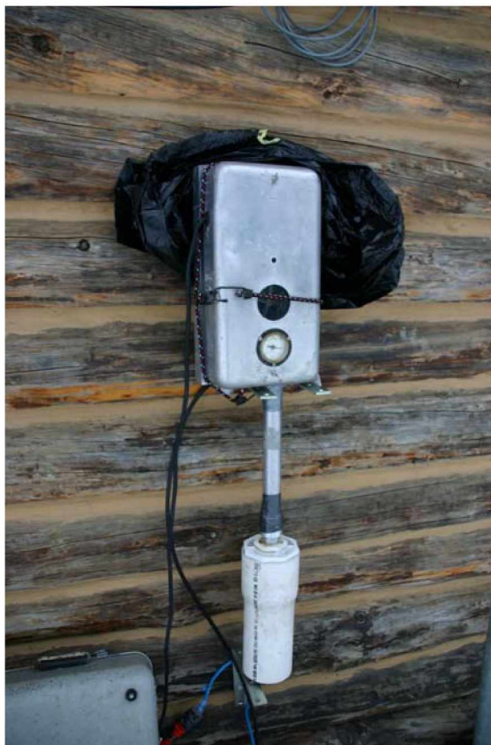
Figure 2.5. The 8-stage DRUM impactor installed at the University of Alaska Homer, AK Field Station. The sampler was inverted from its normal deployment configuration and was fitted with a special inlet (white pipe) for collecting 35.0 \mu\text{m} \text{O}_A and smaller aerosol.
