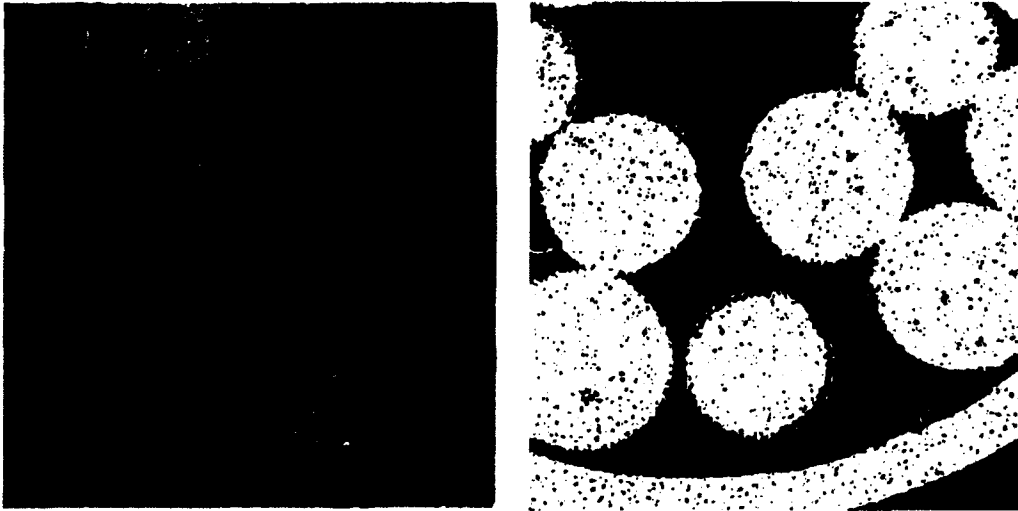
Figure 3.5: Reconstruction of PMMA particles with moisture present. The beam hardening at the edges of the particles and pendular rings, and noise inside the particles, show the same absorption strength as the water and renders the reconstruction useless from a computational point of view.
