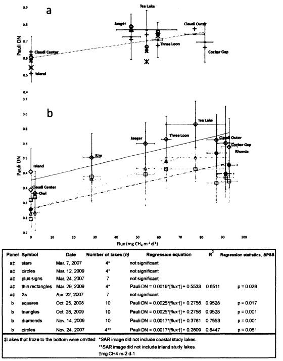
Figure 2.8: Pauli Band 3 roughness component of L-band PALSAR quad-polarized SAR backscatter from thermokarst lake ice, plotted against long-term (120 day) seasonal CH<sub>4</sub> flux for a) spring and b) fall. Error bars show +/- one standard deviation. Note different scales with higher spring SAR values.
