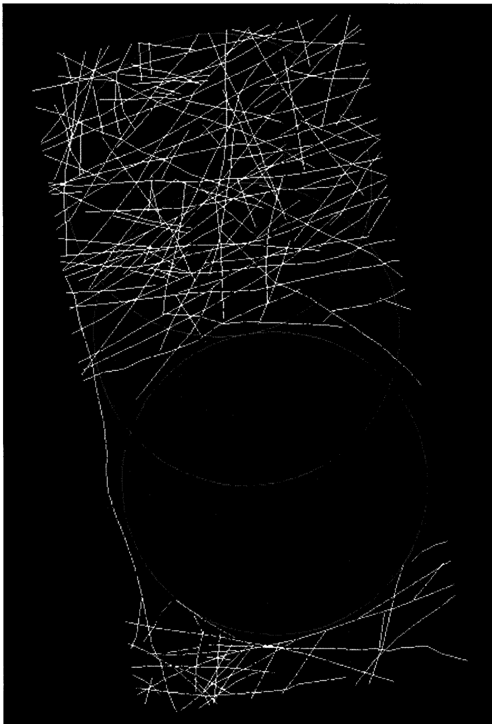
Figure 1.3: Example of the orientation analysis selection process. Here all ELFs (white lines) found in the bottom circle are selected (grey).
