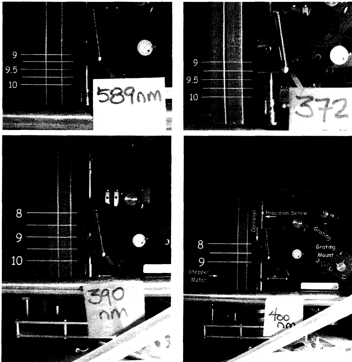
Figure 6.13 Dye laser grating position at four different wavelengths. A carpenter square is placed beside the grating as a reference. (Upper left) Grating at 589 nm with carriage just below 9.25 inch mark. (Upper right) Grating at 372 nm with carriage just below 9.25 inch mark. (Lower left) Grating at 390 nm with carriage just below 9.5 inch mark. (Lower right) Grating at 400 nm with carriage just above 9 inch mark.
