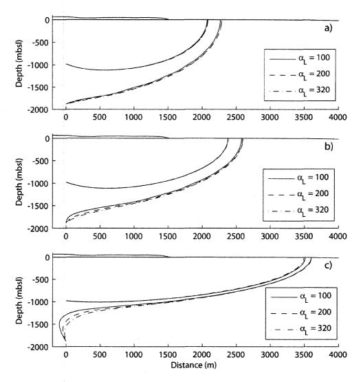
**Figure 7.15** Groundwater travel paths at Cannikin for different dispersivities (100 m, 200 m, and 320 m) and subsurface: a) isotropic, b) anisotropy ratio of 1:2 and c) anisotropy ratio of 1:10. Isotropic subsurface
