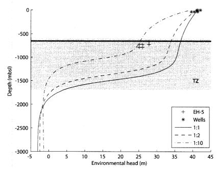
**Figure 7.2** Simulated and measured environmental head measurements at Long Shot (U.S. Corps of Engineers and USGS, 1965). Measured heads are from EH-5 (plus) and shallow wells (star) at the Long Shot test site. Simulated scenarios are isotropic (solid line), anisotropy 1:2 (dashed line) and anisotropy 1:10 (dash dotted line). Thick solid line illustrates the depth of the Long Shot detonation.
