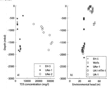
**Figure 3.4** a) Total dissolved salinity (TDS) measurements at Long Shot (EH-5), Cannikin (UAe-1) and Milrow (UAe-2) (Beteem et al., 1971; U.S. Corps of Engineers and USGS, 1965). b) Environmental head measurements at Long Shot (EH-5), Cannikin (UAe-1, UA-1-HTH-1, UA-1), and shallow wells (U.S. Corps of Engineers and USGS, 1965; Ballance, 1972; Ballance and Dinwiddie, 1972;Ballance, 1970).
