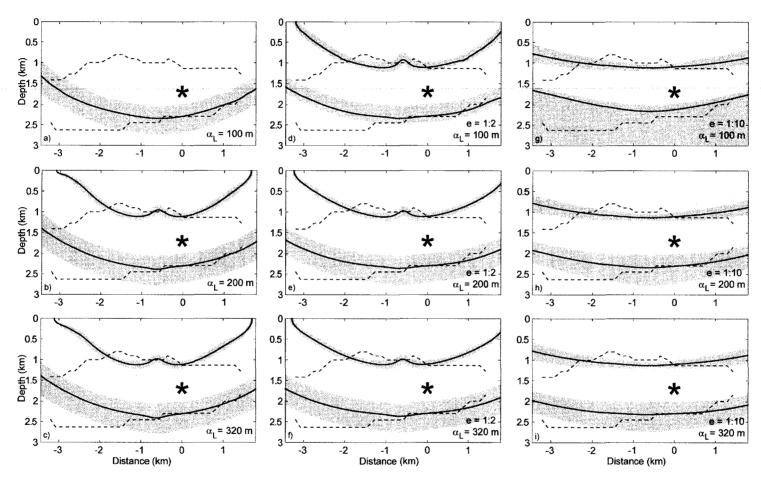
**Figure 7.11** Shapes of the TZ (solid line) for isotropic and anisotropic (e) simulations with different longitudinal dispersivities ( $\alpha_L$ ) at Cannikin (asterisk). The gray field shows the uncertainty range and dashed line is the TZ as estimated by MT (Unsworth et al., 2007). a) shows no top TZ due to the small difference in saltwater concentrations, this is also the reason for the continuous gray field in g).
