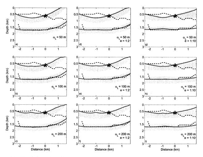
**Figure 7.3** Shapes of the TZ (solid line) at Long Shot for isotropic and anisotropic (e) simulations with different longitudinal dispersivities  $(\alpha_L)$ . The TZ uncertainty range as determined by MT is shown in gray. Dashed line is the TZ as estimated by MT (Unsworth et al., 2007).
