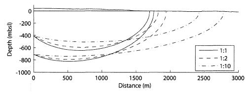
**Figure 7.4** Travel paths at Long Shot for different anisotropy with particles originating at the bottom of the cavity (710 mbsl) and at five cavity radii up into the rubble chimney (410 mbsl). Isotropy is illustrated with a solid line, an anisotropy ratio of 1:2 is illustrated with a dotted line and an anisotropy ratio of 1:10 is illustrated with a dotted-dashed line.
