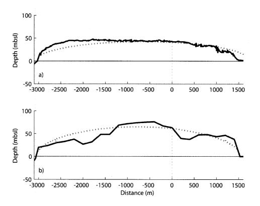
**Figure 7.19** Topography (thick line) and groundwater table (thick dashed line) at a) Long Shot and b) Cannikin when the hydraulic head is not fixed at one meter below the ground surface. The dotted line shows the location of the emplacement hole.
