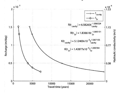
**Figure 7.17** Recharge and hydraulic conductivity plotted versus groundwater travel times with fitted lines for a subsurface with an anisotropy ratio of 1:2 at Cannikin. Particles originate at the bottom of the cavity ( $t_{cavity}$ ) and from five cavity radii up into the rubble chimney ( $t_{sr}$ ) and travels to the seafloor. Longitudinal dispersivity for these simulations is 200 m. The plus illustrates  $t_{cavity}$  and the diamond illustrates  $t_{sr}$  to the seafloor.
