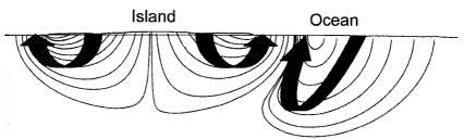
**Figure 3.3** Flow pattern (solid lines) for a homogeneous and isotropic subsurface. The general direction of flow is illustrated with dark gray arrows.
