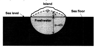
**Figure 3.2** Illustration of island hydrology showing the freshwater lens for a homogeneous subsurface. The thickness of the freshwater lens (z) is approximately forty times the elevation of the groundwater table from the sea level (h).
