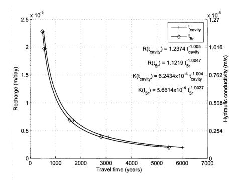
**Figure 7.7** Recharge and hydraulic conductivity plotted versus groundwater travel times with fitted lines for a subsurface with an anisotropy ratio of 1:2 at Long Shot. Particles originate at the bottom of the cavity ( $t_{cavity}$ ) and from five cavity radii up into the rubble chimney ( $t_{5r}$ ) and travel to the seafloor. Longitudinal dispersivity for these simulations is 200 m. The plus symbol illustrates  $t_{5r}$  to the seafloor.
