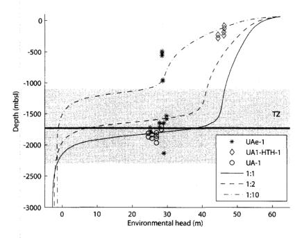
**Figure 7.13** Simulated and measured environmental head measurements at Cannikin. Measured heads are from UAe-1 (plus), UA1-HTH-1 (diamond) and UA-1 (circle). Simulated scenarios (11, 14, 17) with an isotropic subsurface (solid line), anisotropy 1:2 (dashed line) and anisotropy ratio 1:10 (dash dotted line). Thick solid line illustrates the depth of the Cannikin detonation.
