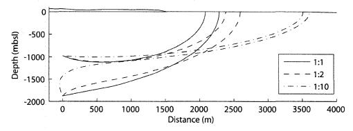
**Figure 7.14** Travel paths at Cannikin for particles originating at the bottom of the cavity (1,880 mbsl) and at five cavity radii up into the rubble chimney (980 mbsl). Isotropic is illustrated with a solid line, an anisotropy ratio of 1:2 is illustrated with a dotted line and an anisotropy ratio of 1:10 is illustrated with a dotted-dashed line.
