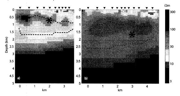
**Figure 3.5** Electrical resistivity models of the a) Long Shot and b) Cannikin profile derived from magnetotelluric (MT) data (Unsworth, 2007). The triangles show locations of MT measurement stations and asterisks show the nuclear explosion locations. Dashed lines illustrate the TZ and are associated with a downward decrease in resistivity caused by an increase in groundwater salinity (Unsworth et al., 2007).
