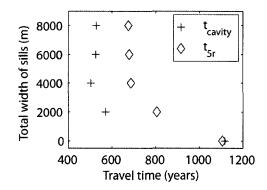
**Figure 7.9** Total width of sills plotted versus groundwater travel times for the andesite sill layer simulations at Long Shot. A plus illustrates the groundwater travel time from the bottom of the cavity ( $t_{cavity}$ ) and diamond illustrates the groundwater travel time from five cavity radii up into the rubble chimney ( $t_{5r}$ ) to the seafloor.
