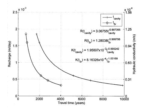
**Figure 7.16** Recharge and hydraulic conductivity plotted versus groundwater travel times with fitted lines for an isotropic subsurface at Cannikin. Particles originate at the bottom of the cavity  $(t_{cavity})$  and from five cavity radii up into the rubble chimney  $(t_{5r})$  and travels to the seafloor. Longitudinal dispersivity for these simulations is 200 m. The plus illustrates  $t_{cavity}$  and the diamond illustrates  $t_{5r}$  to the seafloor.
