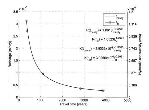
**Figure 7.6** Recharge and hydraulic conductivity plotted versus groundwater travel times with fitted lines for an isotropic subsurface at Long Shot. Particles originate at the bottom of the cavity  $(t_{cavity})$  and from five cavity radii up into the rubble chimney  $(t_{5r})$  and travel to the seafloor. Longitudinal dispersivity for these simulations is 200 m. The plus symbol illustrates  $t_{cavity}$  and the diamond illustrates  $t_{5r}$  to the seafloor.
