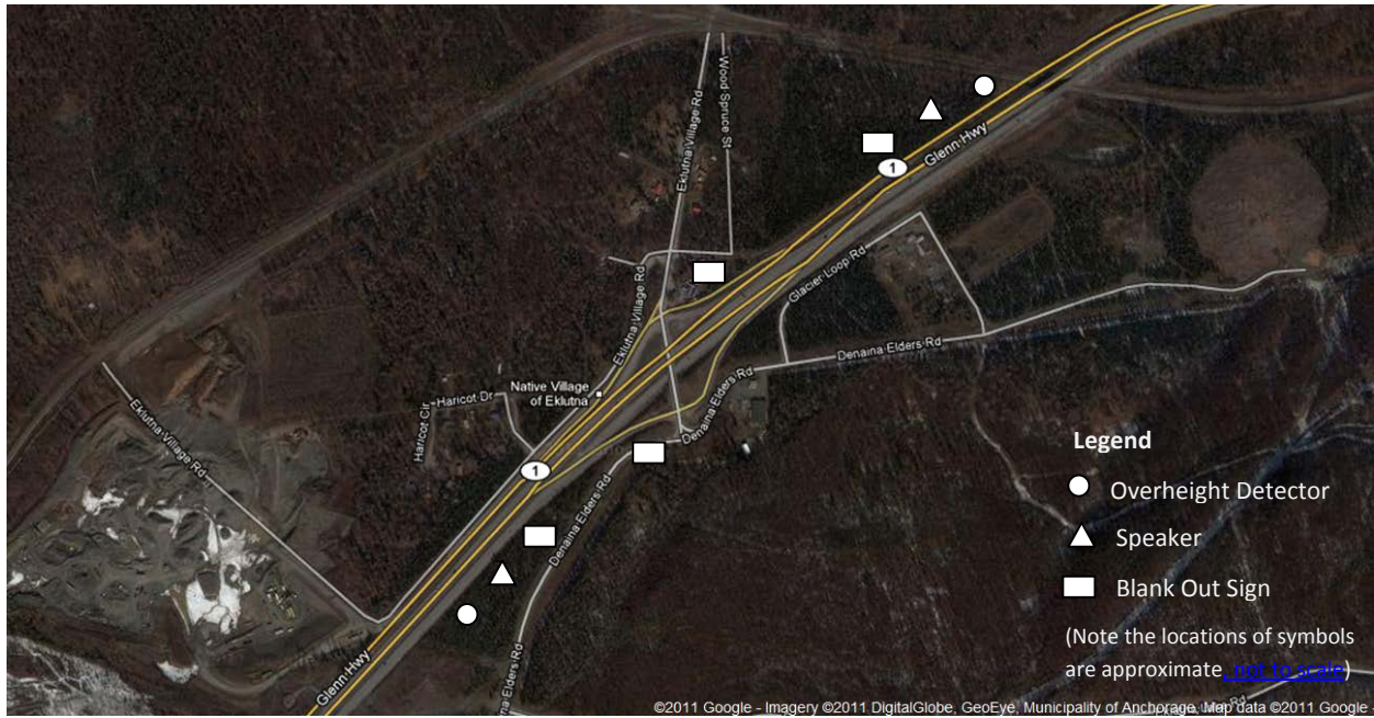
Figure 1 The Location of the Original Eklutna Overhead Detection System
