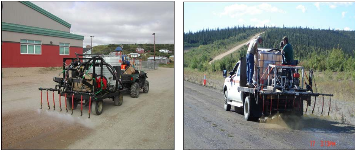
Figure 12. Low-cost synthetic fluid applicators
