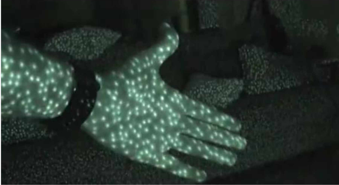
FIGURE 5: IR DOT PATTERN EMITTED BY THE KINECT
