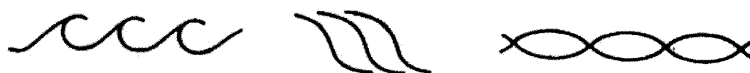
FIG. 4.1. Schematic views of three patterns commonly observed: billow (left), braids (middle), and cat's eye (right) (Gossard and Hooke 1975).
