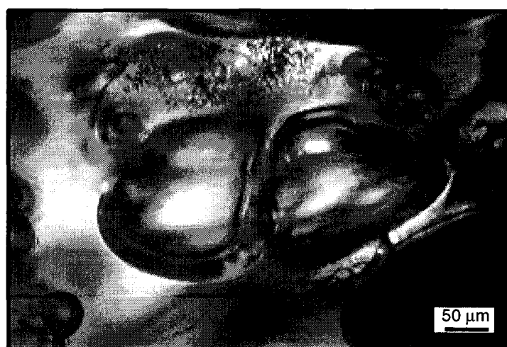
Figure 1.9 Typical bubble pair shortly before coalescence. Note the planar shape of the thin separation wall between the bubbles (G303, Table 1.2).
