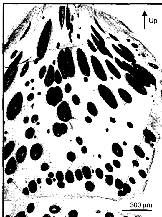
Figure 1.8 Reflected light microphotograph of an open degassing run showing the catalyzing effect of shear on coalescence. Note that the large, coalesced bubbles are restricted to the upper half of the photograph. The photograph corresponds to the upper 2 mm of the sample (G318, Table 1.2).
