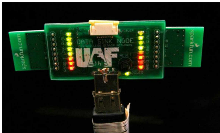
Figure 3-10: Data Sink for Relaying Data from the Wireless Medium to the Computer
