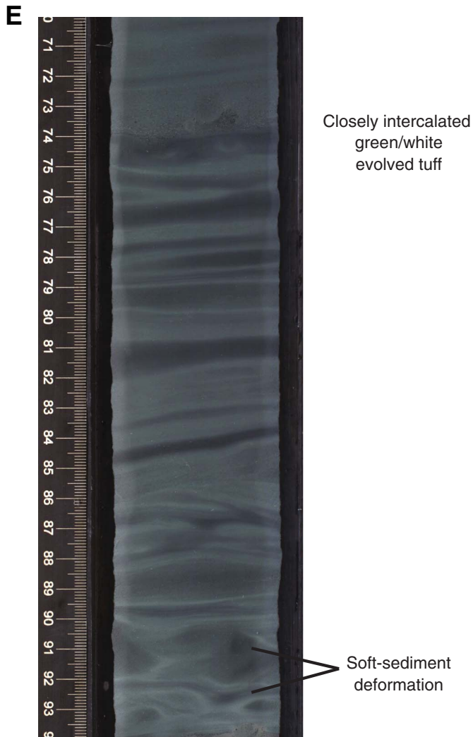
Figure F30 (continued). E. Closely intercalated green and white evolved very fine grained tuff with soft-sediment deformation (58R-3, 70–94 cm; 964.16–964.40 mbsf).
