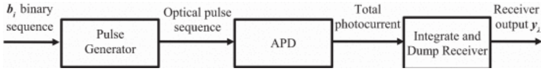
Fig. 1: A schematic diagram of an OOK optical communication system employing an APD-based integrate and dump receiver.
