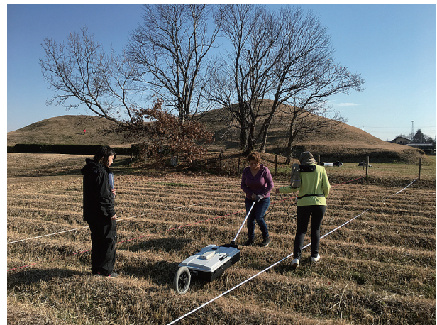
Plate 4 Operating GPR on surrounding moat (inner)
