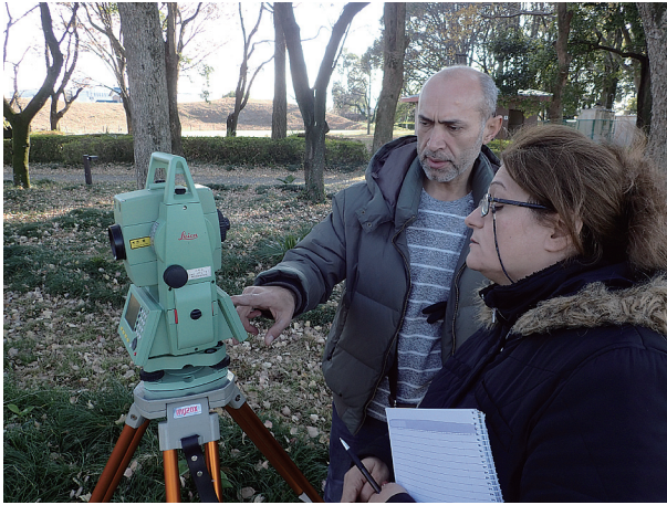
Plate 1 Measuring reference points with TS
