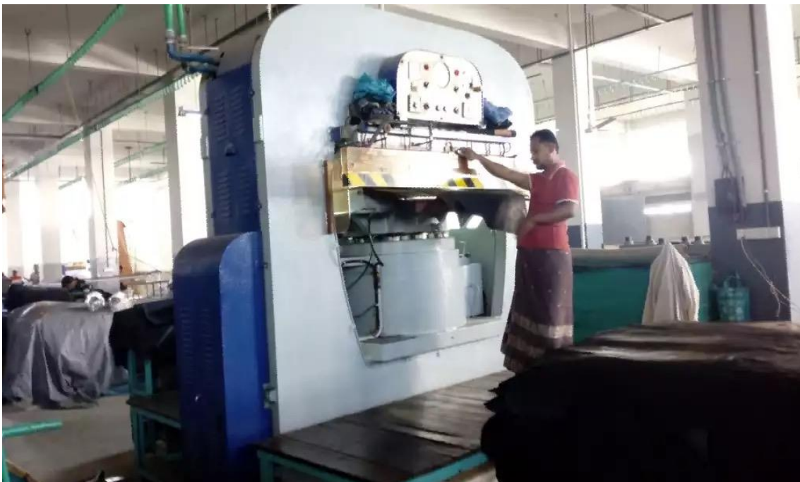
Fig. 2.10 Hydraulic press machine to emboss the leather
