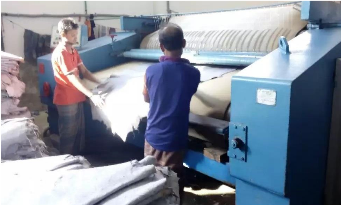
Fig. 2.6 Mechanical samming of pelts
