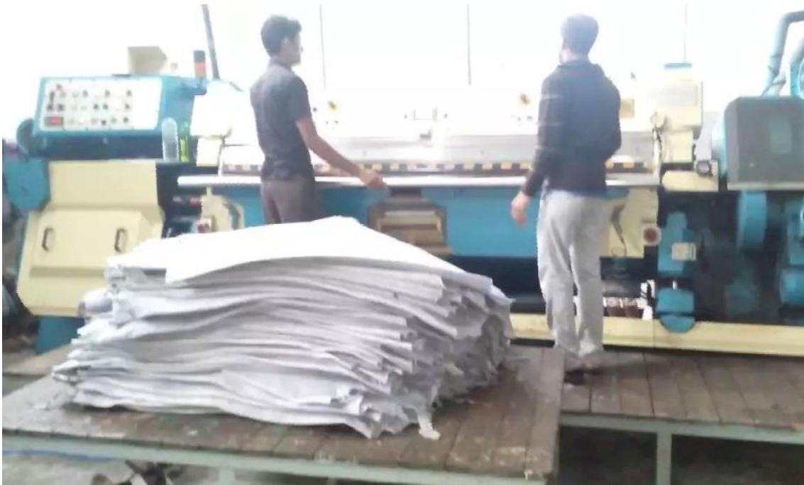
Fig. 2.7 Mechanical splitting of pelts
