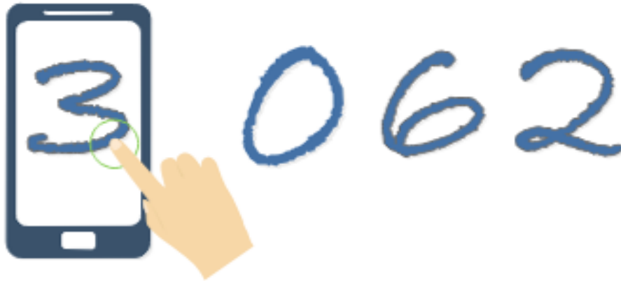
Fig. 1.1 How PINWrite system works on smartphone: users are asked to write their password on the screen one by one instead of typing the keyboard.
