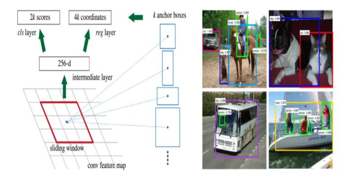
Fig. 7 RPN framework and examples detection using RPN (from [5])
