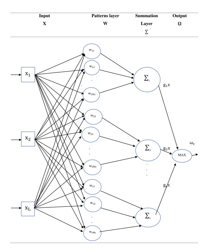
Fig. 1 Architecture for the Probabilistic Neural Network
