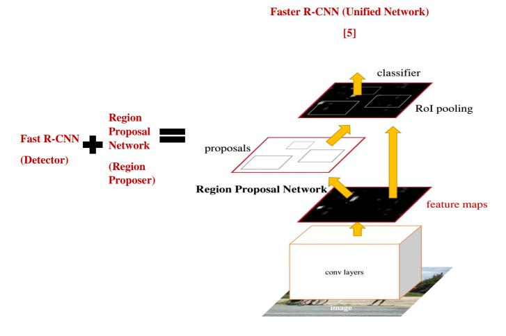
Fig. 6 Faster R-CNN as a single, unified network for objection detection
