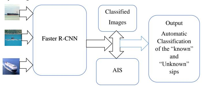
Fig. 21 Faster R-CNN-AIS conceptual model
