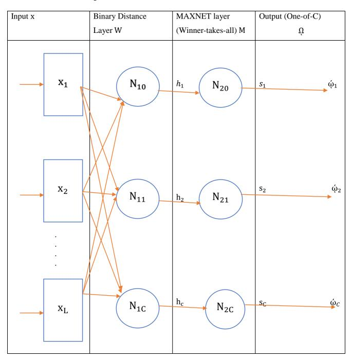
Fig. 2 Architecture for the Hamming Neural Network
