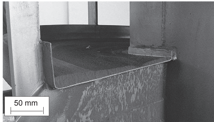
Figure 1.25 Photograph of particle layers transported by the outlet of a spiral elevator; obtained from literature [71].
