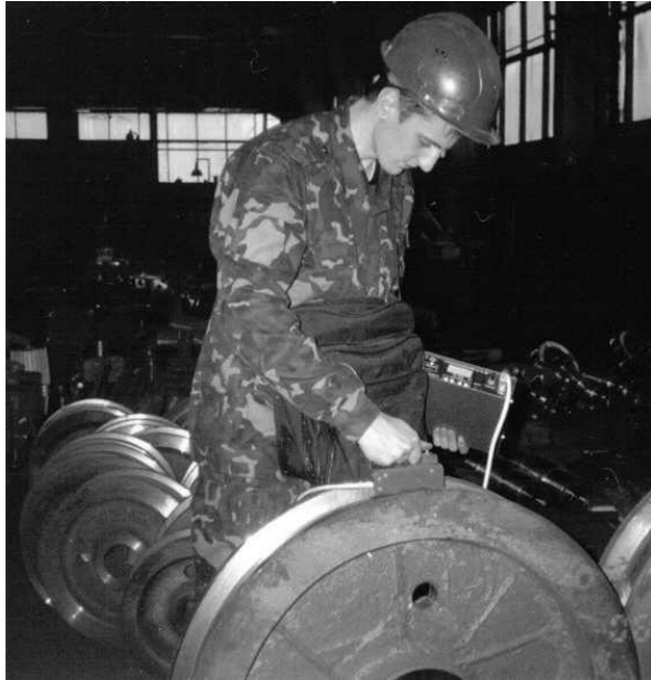
Figure 1. Carrying out the magnetic method of nondestructive control (NC) on crane wheels
