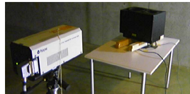
Fig.7. Picture of experiment. The loudspeaker is located on the table toward the ceiling.
