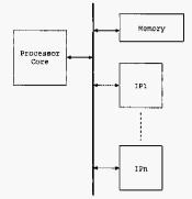
Fig. 2. An architecture model of IP-based SoC ,
