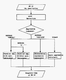
Fig. 7. A response time calculation flow.
