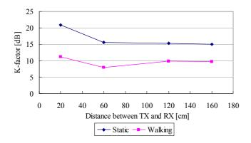
Figure 6. The measured K-factor when static and walking test conditions.
