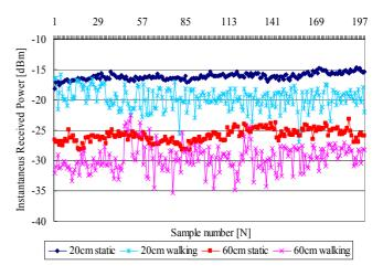
Figure 5. Received instantaneous power over 200 samples when distance between TX and RX is 20cm and 60cm and test person is static and moving.
