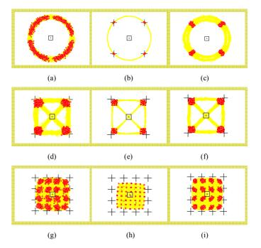
Figure 7. Constellation diagram results: (a) MSK air channel SR=500Ksps & DTR=90cm, (b) MSK intra-body channel SR=500Ksps & DTR=90cm, (c) MSK intra-body channel SR=1Msps & DTR=180cm, (d) QPSK air channel SR=500Ksps & DTR=90cm, (e) QPSK intra-body channel SR=500Ksps & DTR=90cm, (f) QPSK intra-body channel SR=1Msps & DTR=180cm, (g) 16QAM air channel SR=500Ksps & DTR=90cm, (i) 16QAM intra-body channel SR=500Ksps & DTR=90cm, (i) 16QAM intra-body channel SR=1Msps & DTR=180cm.
