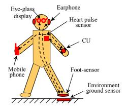
Figure 1. Example scenario of BAN devices distribution
