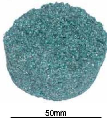
Fig. 3-1 SiC Preform before infiltration process
