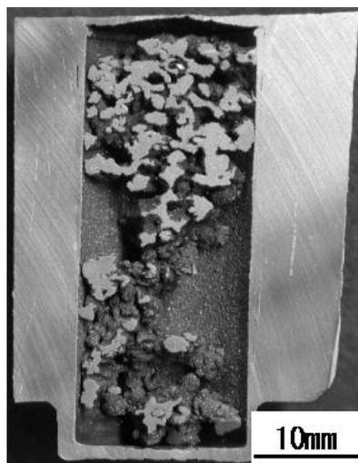
Fig. 5-13 Cross section of DRA produced using polished case with glass shot
