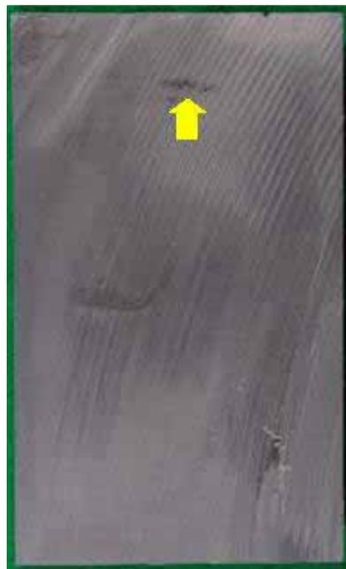
Fig. 4-6 Cross section of preform with NiO powder and Ar bubbling process. (infiltration ratio: 99.5%)
