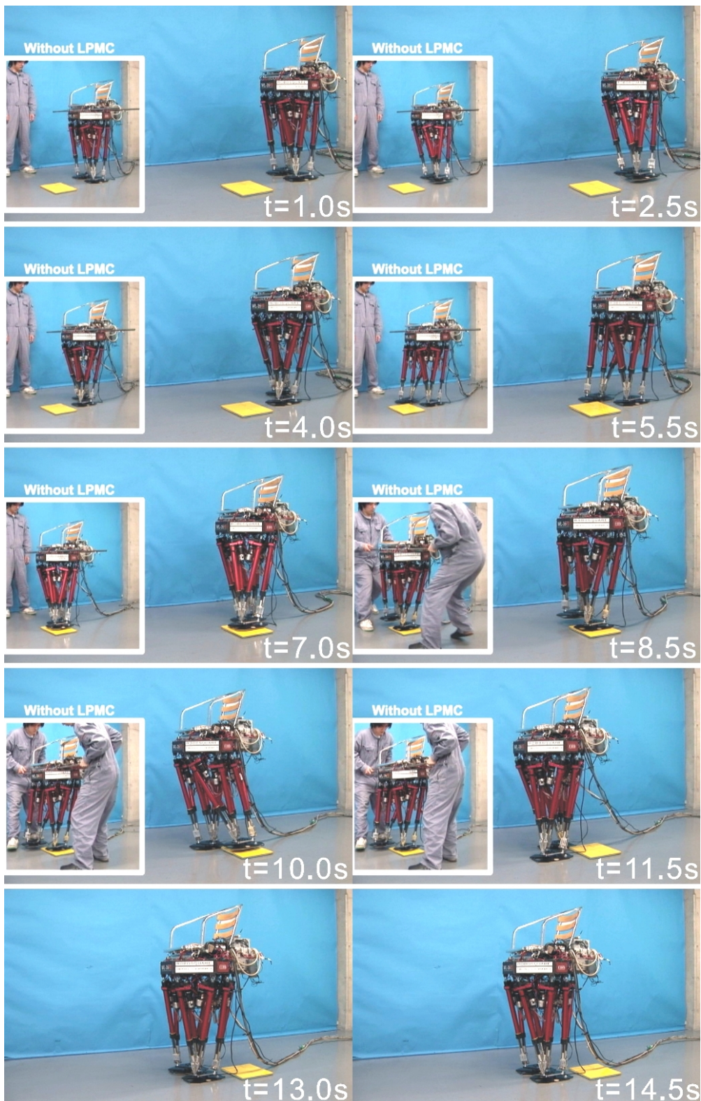
Figure 3.9 Walking experiment, stepping on 20 mm board along the z axis. (Walking forward, walking cycle: 2.0 s/step, step length: 200 mm/step, height of unevenness: 20 mm)
