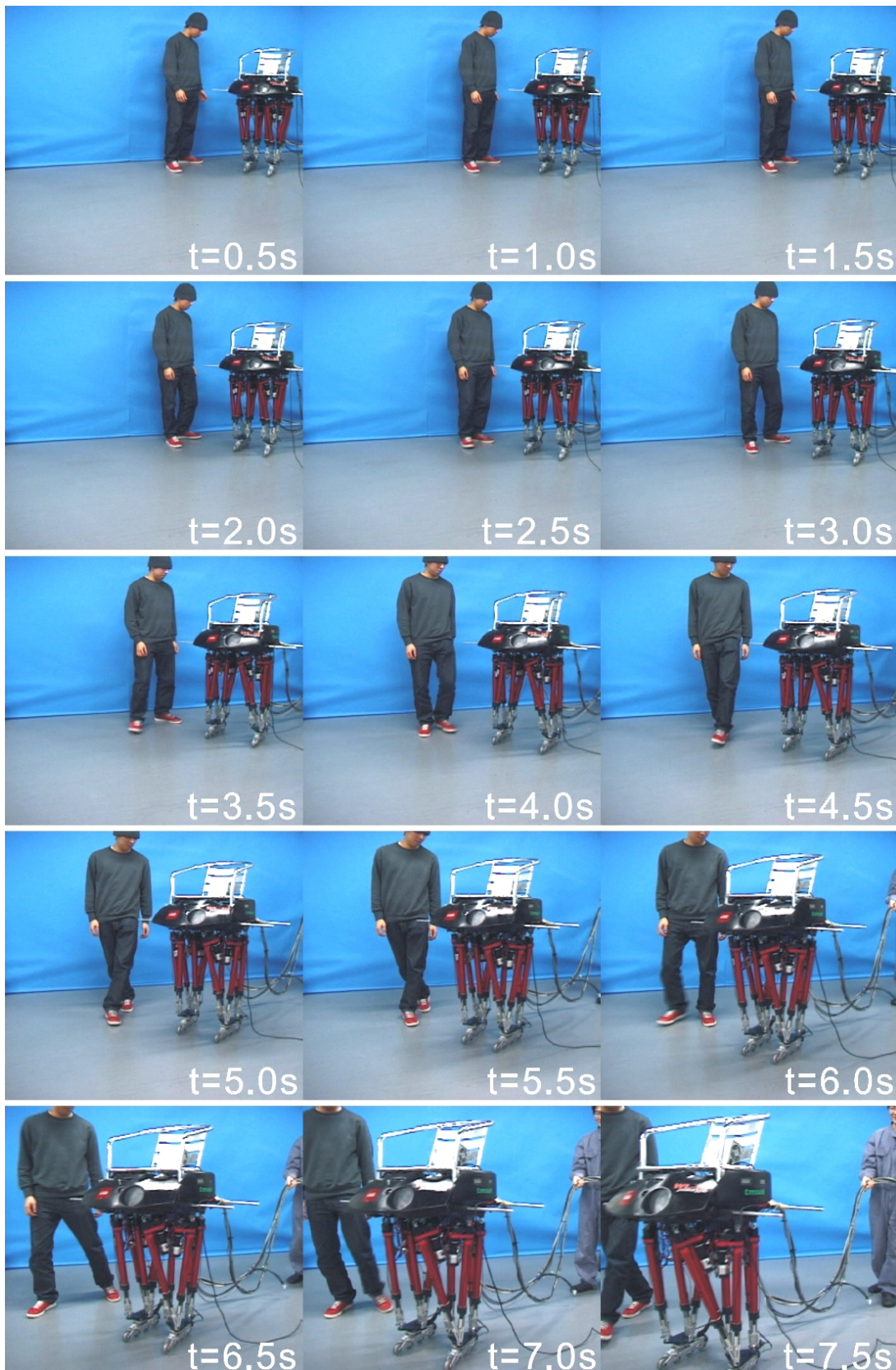
Figure 6.7 Skating experiments using inline skate system, WS-3.
