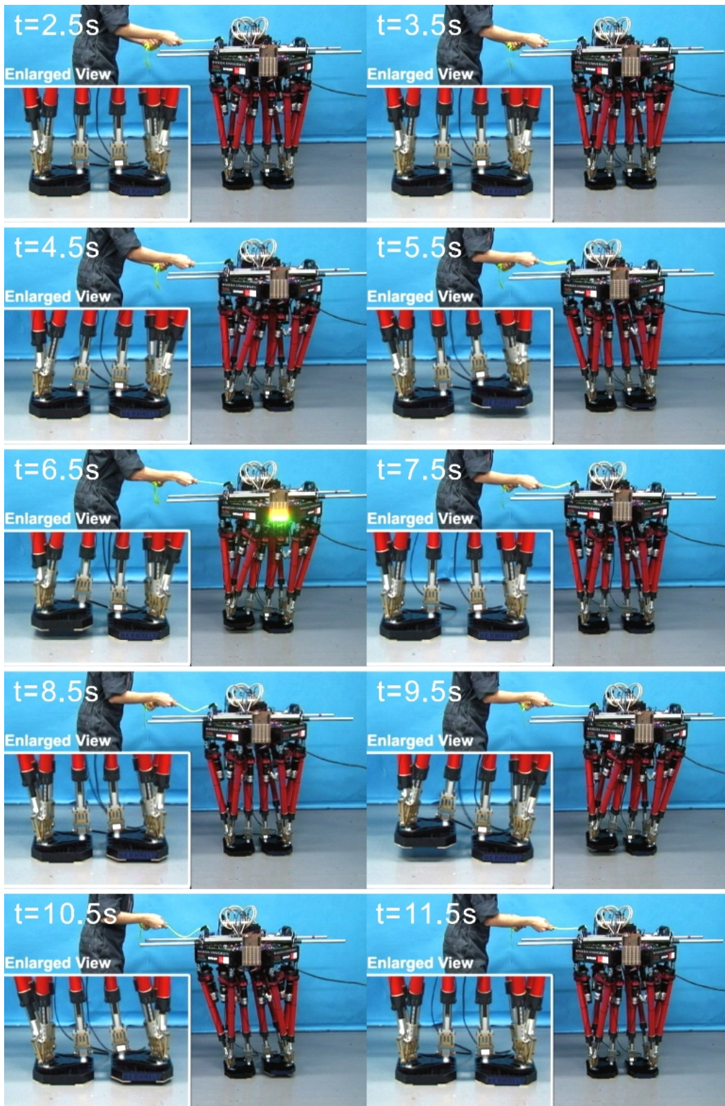
Figure B.14 Walking experiment, pulling the robot rightward at the third step. (Stamping, walking cycle: 0.8 s/step)
