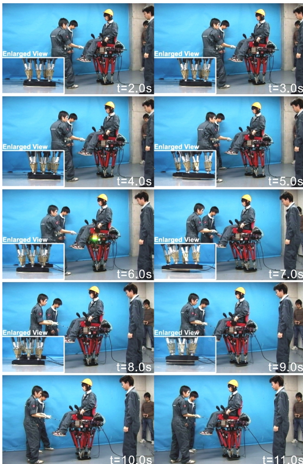
Figure B.49 Walking experiment, pulling the robot forward at the third step. (Walking forward, walking cycle: 1.0 s/step, step length: 100 mm/step, load: a 50 kg human)
