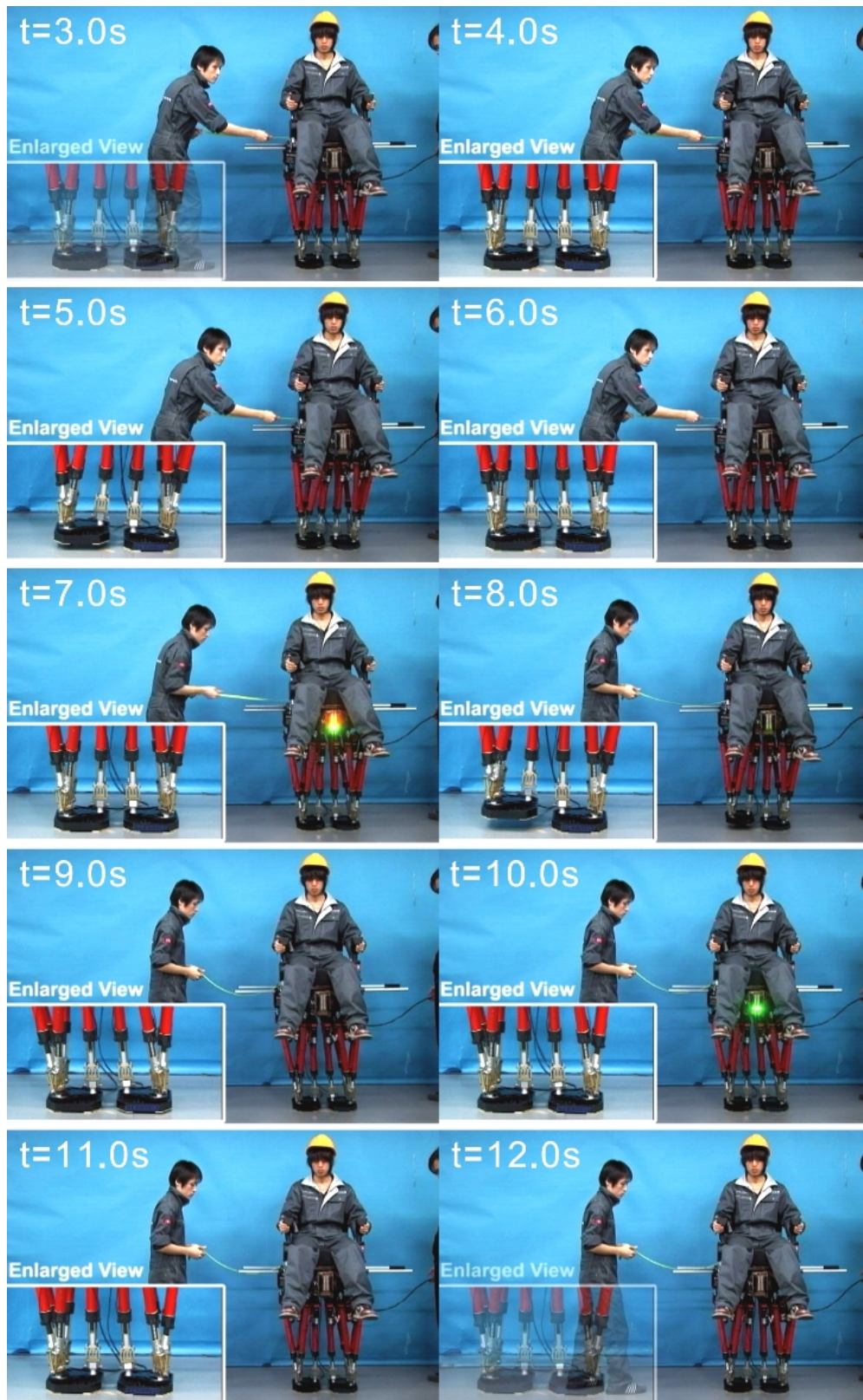
Figure B.44 Walking experiment, pulling the robot rightward at the third step. (Stamping, walking cycle: 0.8 s/step, load: a 50 kg human)
