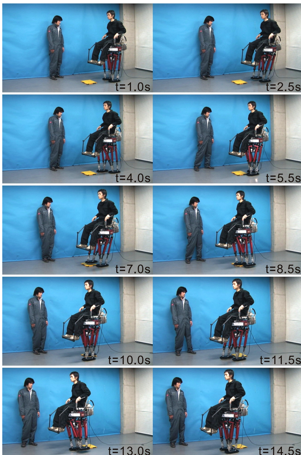
Figure A.24 Walking experiment on 20 mm board, carrying a human. (Walking forward, walking cycle: 2.0 s/step, step length: 200 mm/step, height of unevenness: 20 mm, load: a 55 kg human)
