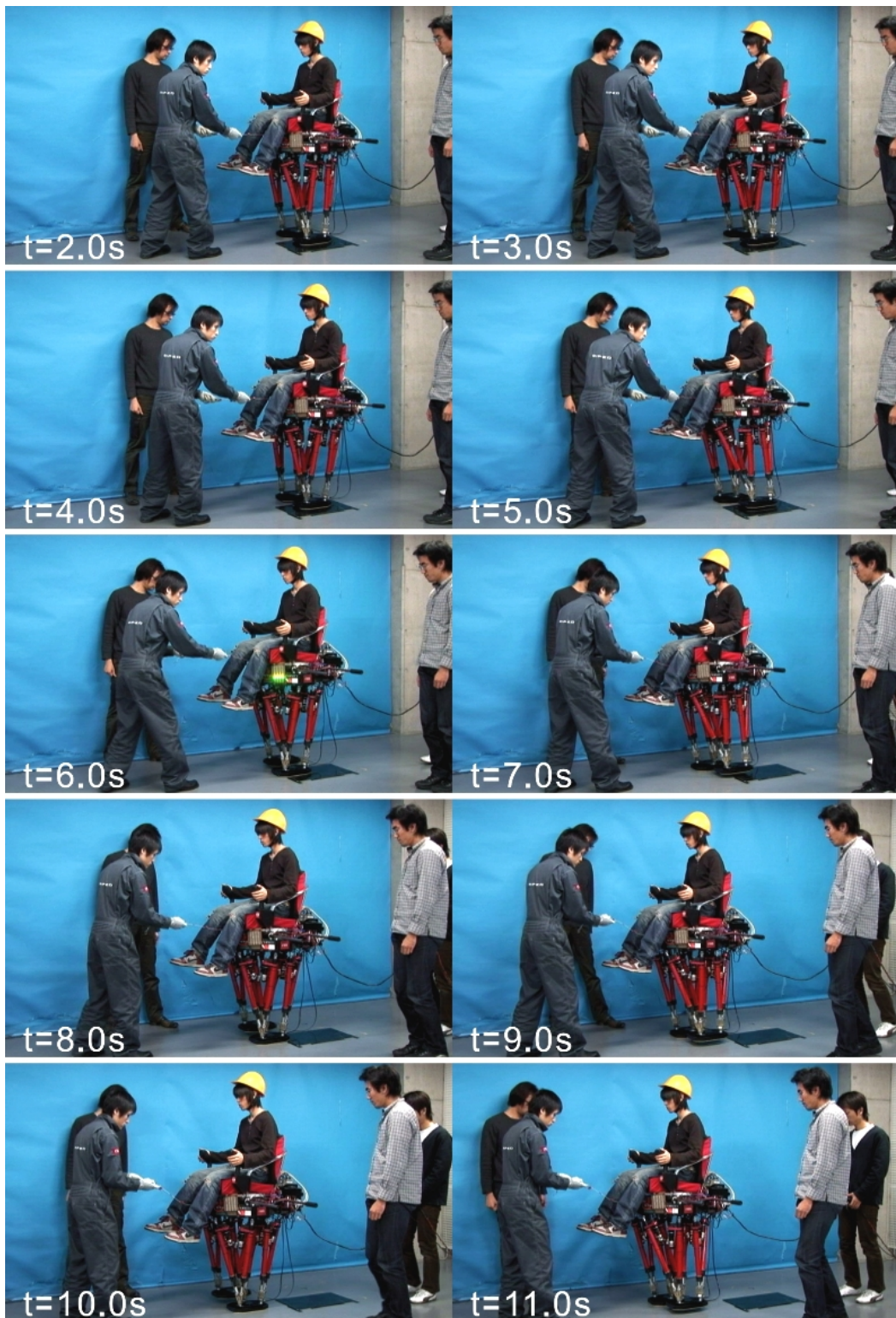
Figure B.64 Walking experiment, stepping down 5 mm board and pulling the robot forward at the third step.
