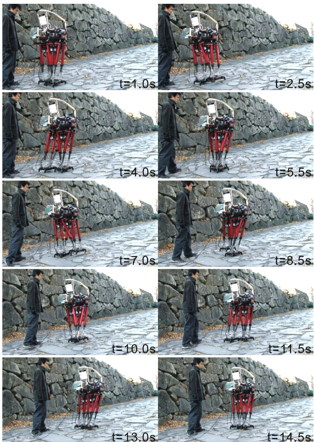
Figure 4.14 Walking experiment on uneven terrain with 20 mm height and 10 deg inclination. The robot's feet are WS-1R adaptable to uneven terrain. (Walking forward, walking cycle: 2.0 s/step, step length: 200 mm/step, height of unevenness: 20 mm, inclination: 10 deg)
