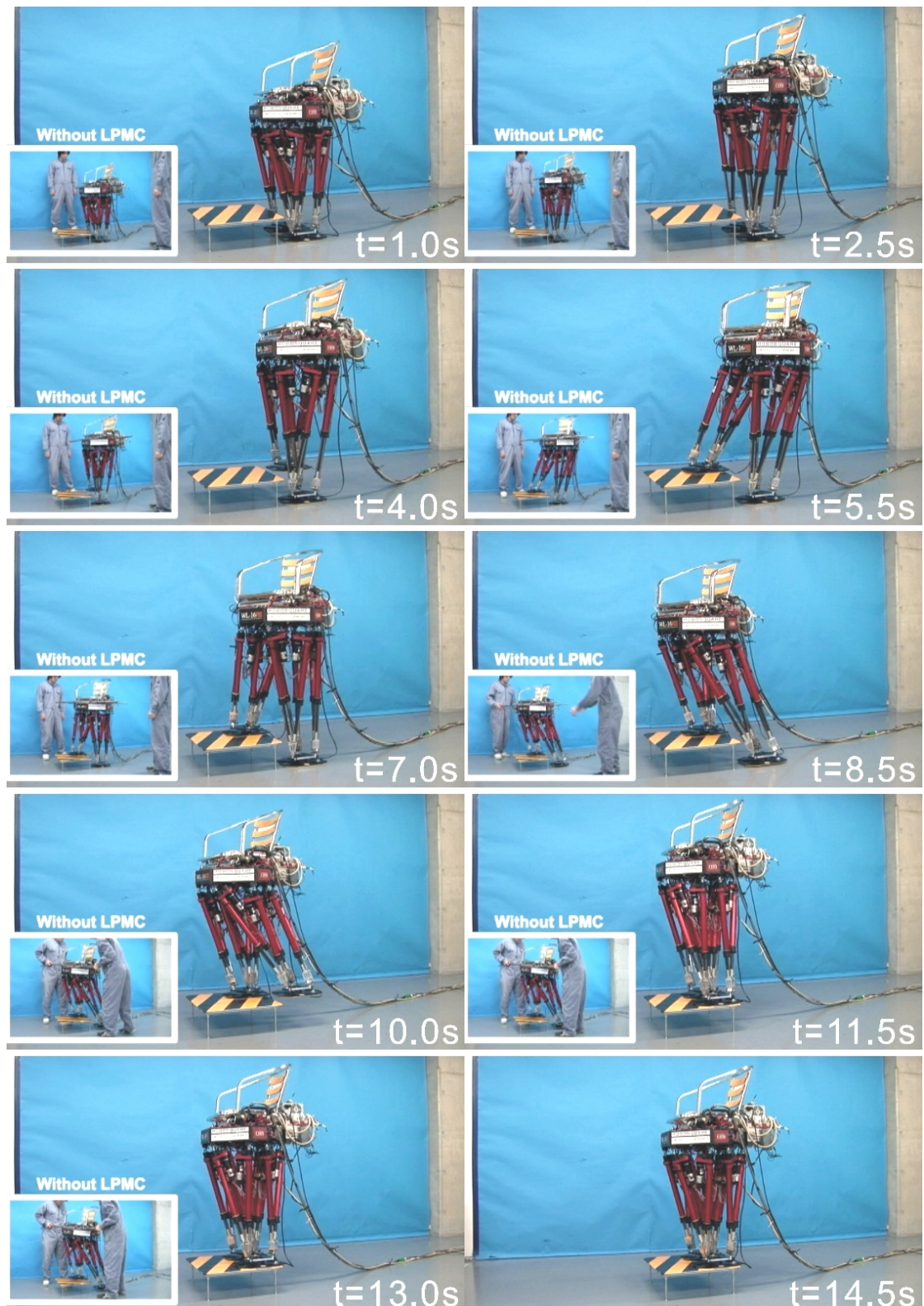
Figure 3.24 Walking experiment in ascending a stair. The preset stair height in the reference walking pattern is 150 mm, while the measured stair height is 170 mm. The walking cycle is 5.8 s/step.
