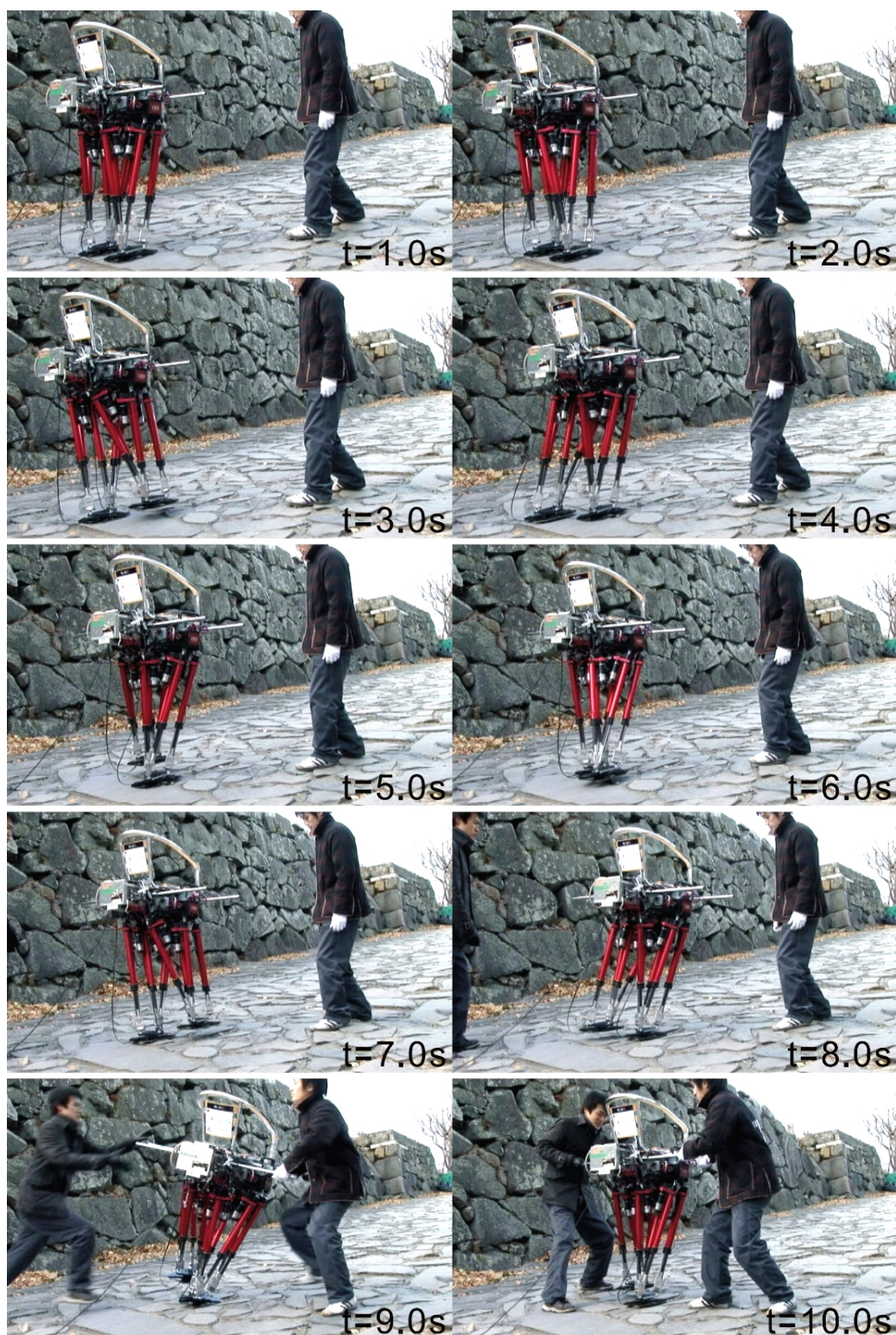
Figure 4.13 Walking experiment on uneven terrain with 20 mm height and 10 deg inclination. The robot's feet are rigid, flat soles.
