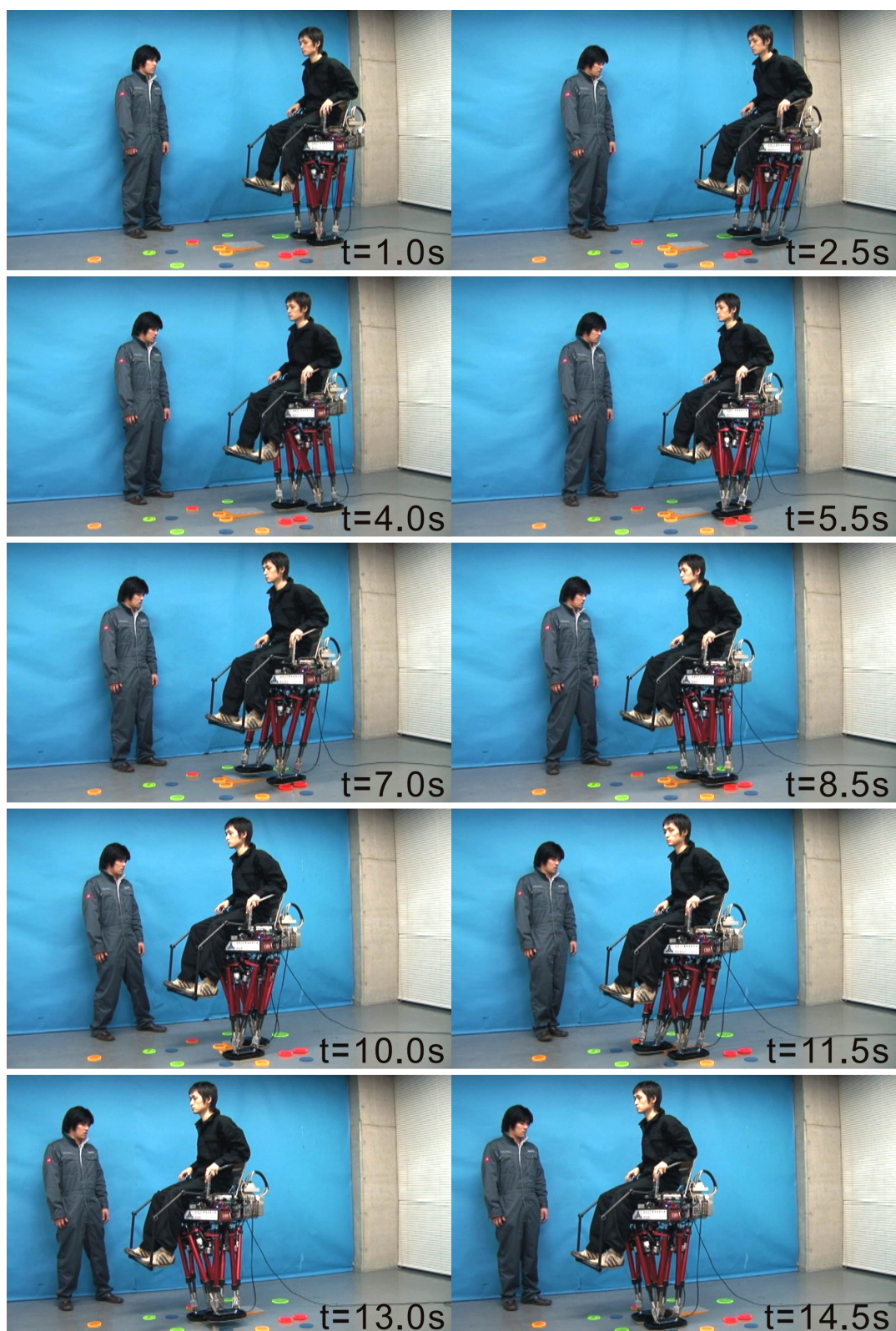
Figure A.28 Walking experiment on uneven surface, carrying a human. (Walking forward, walking cycle: 2.0 s/step, step length: 200 mm/step, height of unevenness: 5-20 mm, load: a 55 kg human)
