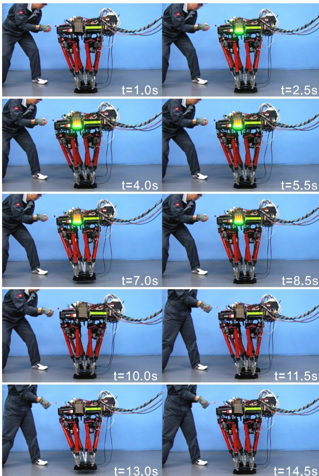
Figure B.85 Walking experiment, pulling the robot forward and suddenly quitting hold of the wire.
