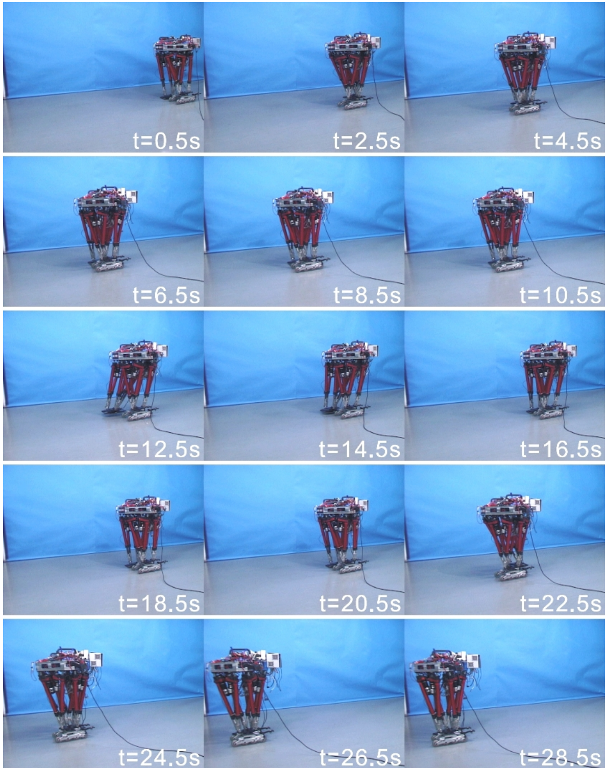
Figure 7.12 Skating experiments using roller skate system, WS-4.
