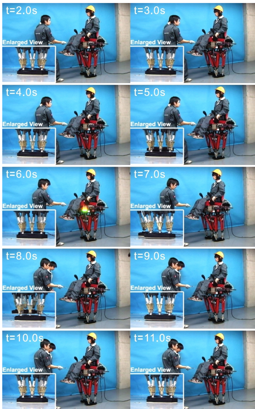
Figure B.39 Walking experiment, pulling the robot forward at the third step. (Stamping, walking cycle: 0.8 s/step, load: a 50 kg human)
