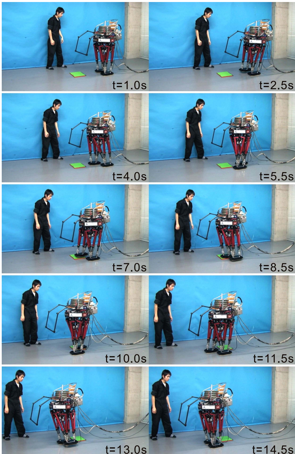
Figure A.20 Walking experiment on 15 mm board, carrying 50 kg load. (Walking forward, walking cycle: 2.0 s/step, step length: 200 mm/step, height of unevenness: 15 mm, load: 50 kg)
