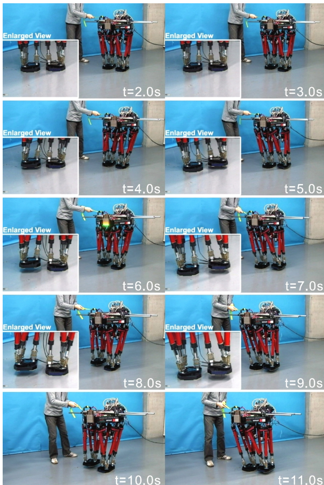
Figure B.19 Walking experiment, pulling the robot rightward at the third step. (Walking forward, walking cycle: 1.0 s/step, step length: 100 mm/step)
