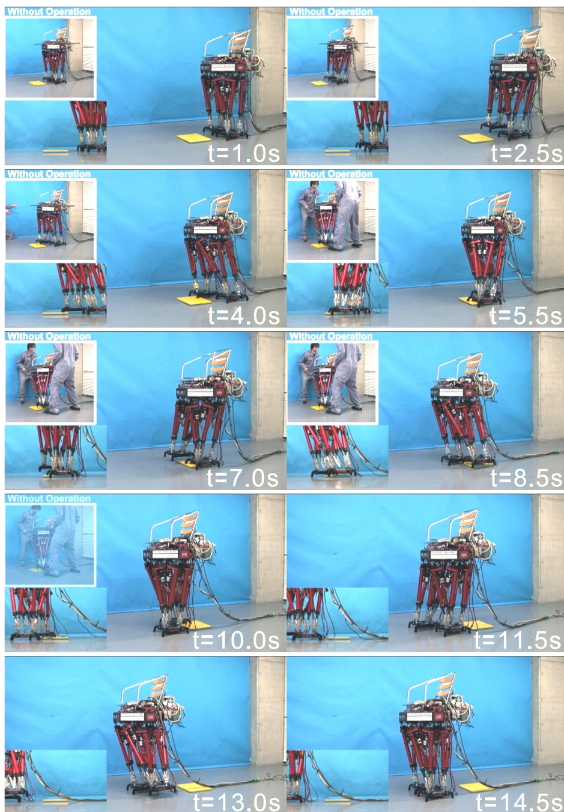
Figure 2.15 Walking experiment on 20 mm board when WS-1R was operated. (Walking forward, walking cycle: 2.0 s/step, step length: 200 mm/step, height of unevenness: 20 mm)
