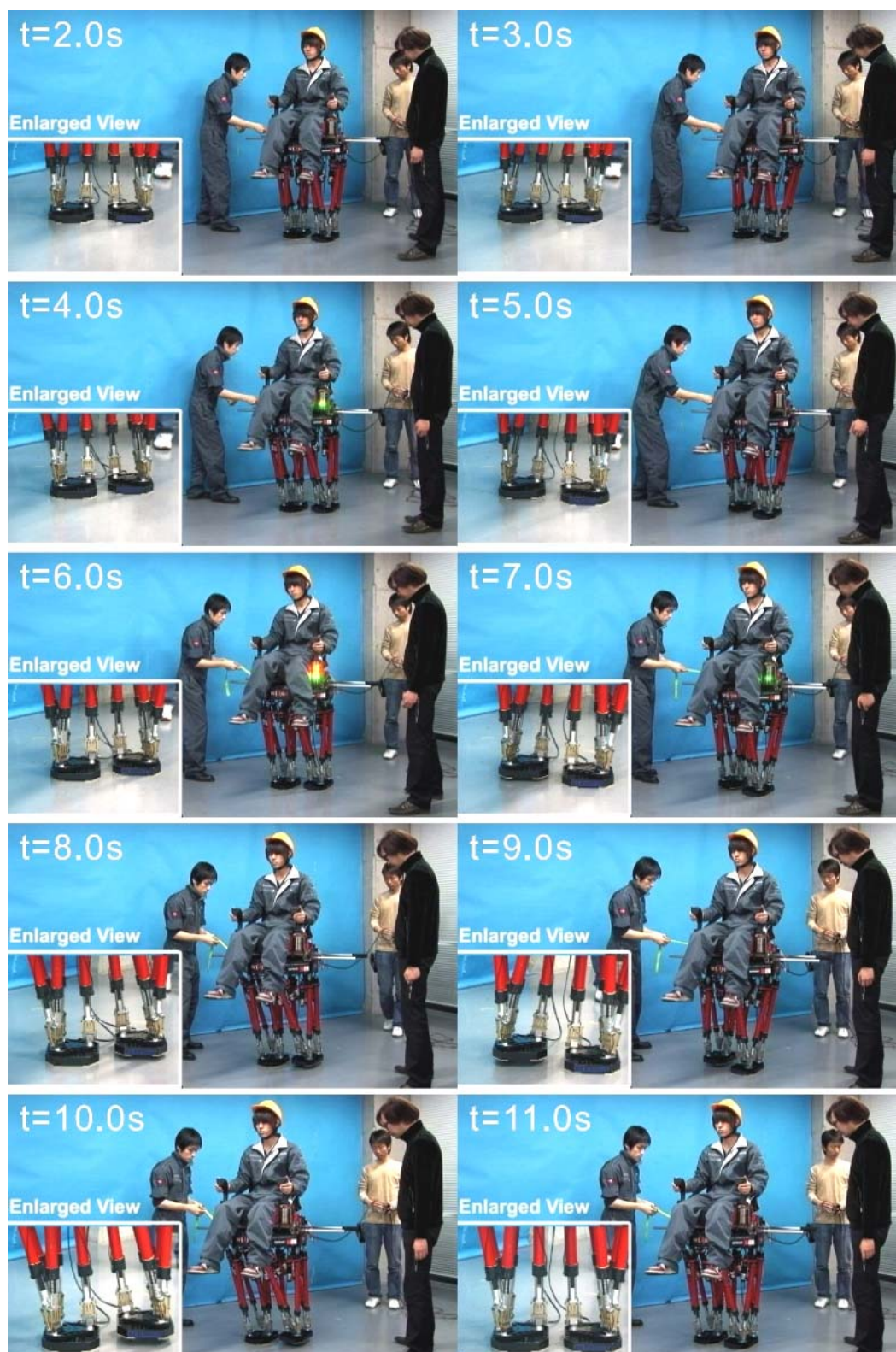
Figure B.54 Walking experiment, pulling the robot rightward at the third step. (Walking forward, walking cycle: 1.0 s/step, step length: 100 mm/step, load: a 50 kg human)
