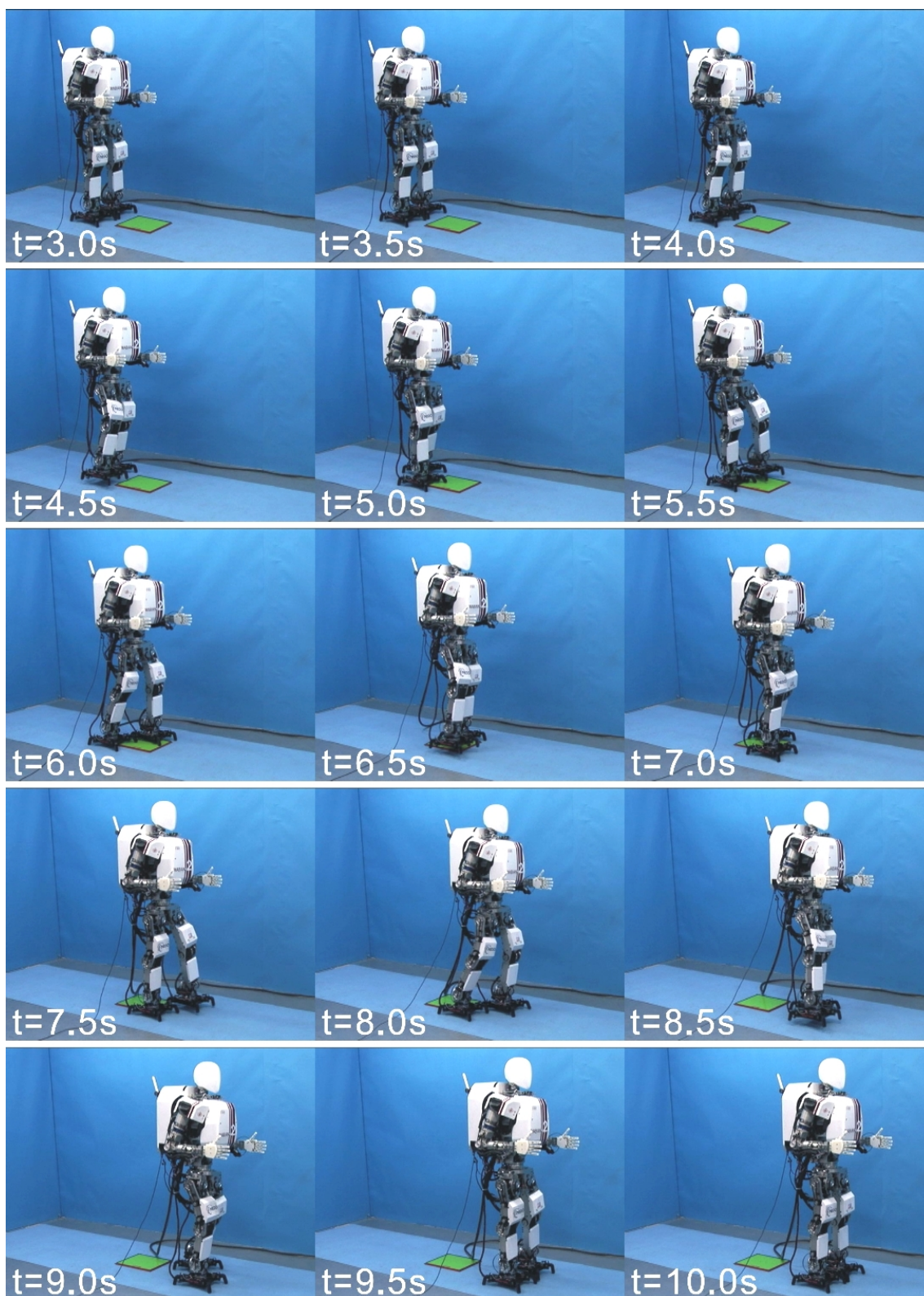
Figure 2.27 Walking experiment using WABIAN-2R mounted on WS-1R. (Walking forward, walking cycle: 1.0 s/step, step length: 200 mm/step, height of unevenness: 20 mm)
