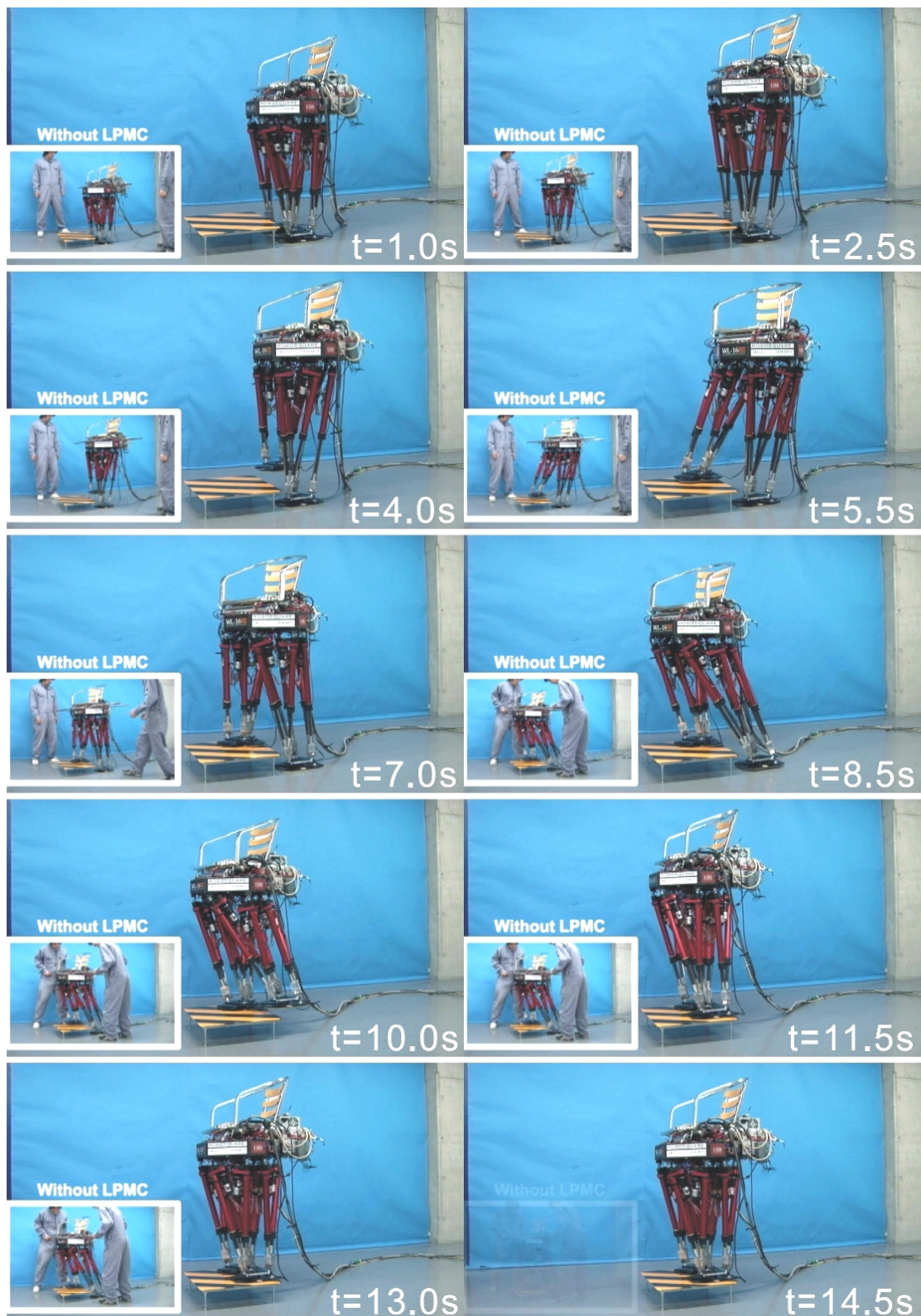
Figure 3.21 Walking experiment in ascending a stair. The preset stair height in the reference walking pattern is 150 mm, while the measured stair height is 130 mm. The walking cycle is 5.8 s/step.
