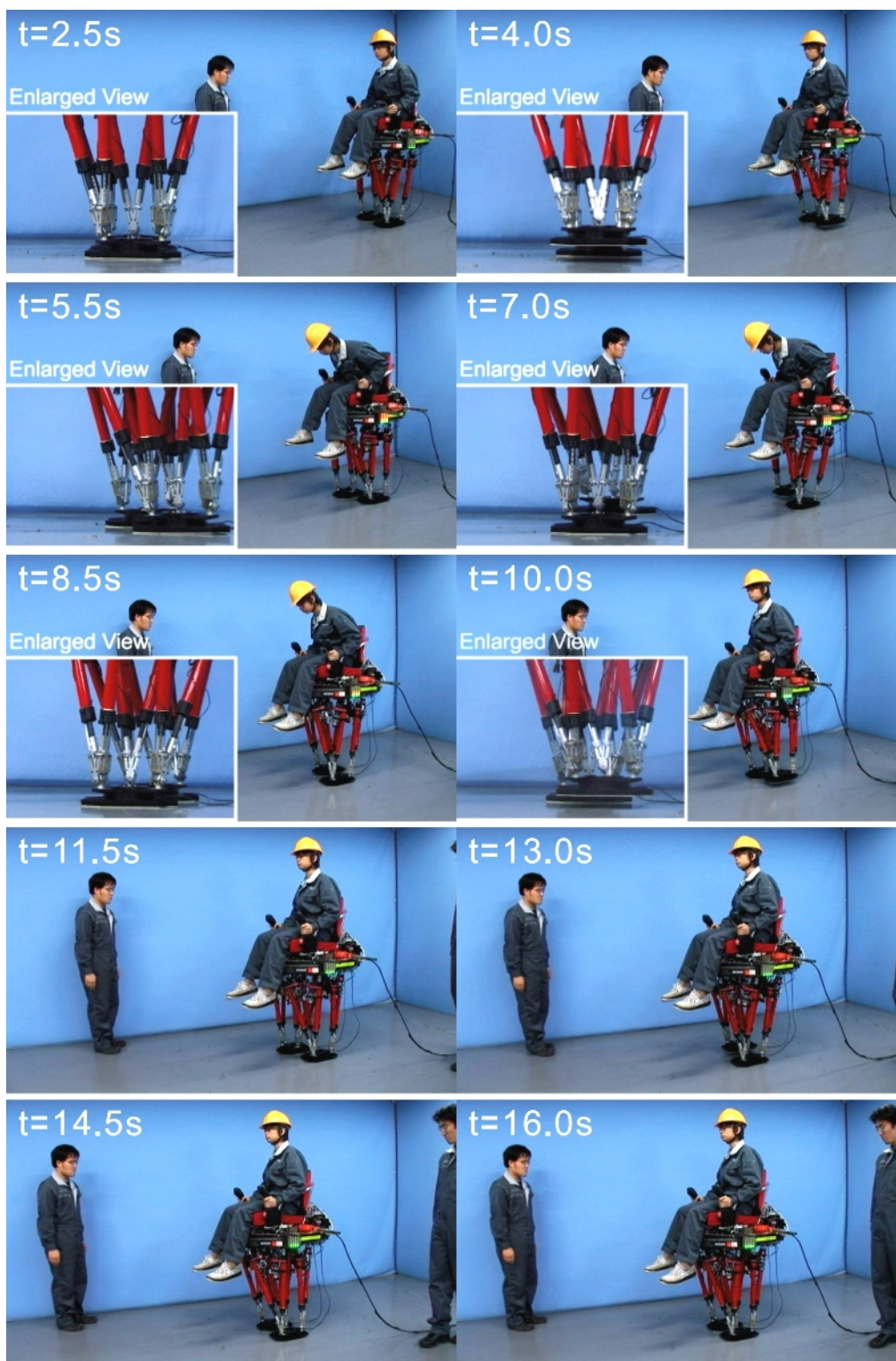
Figure B.90 Walking experiment, carrying a human. A human bent down suddenly during walking.
