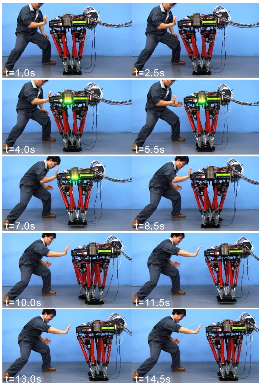
Figure B.97 Walking experiment under external force from environments. (Stamping, walking cycle: 1.0 s/step)
