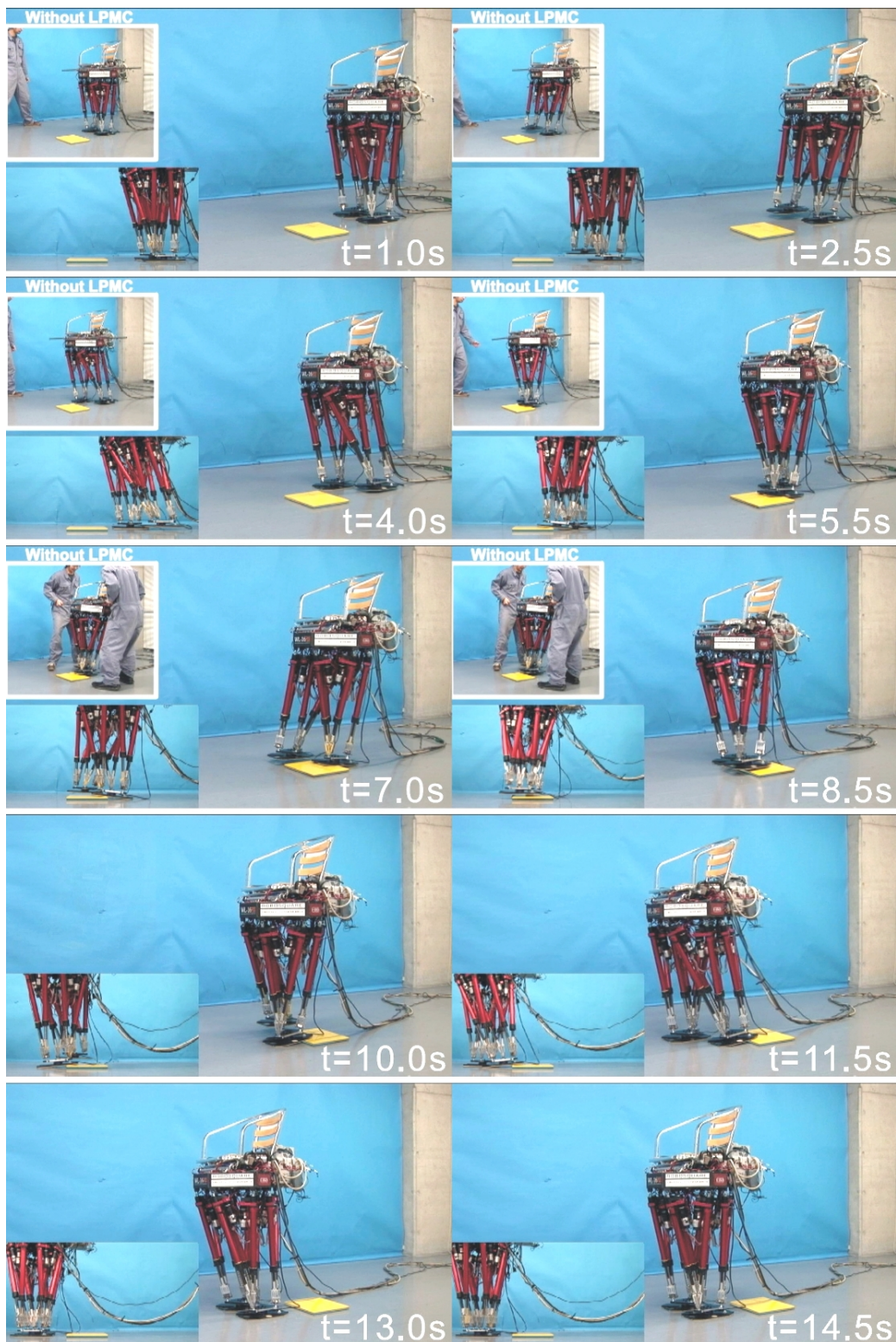
Figure 3.12 Walking experiment, stepping on 20 mm board about the pitch axis. (Walking forward, walking cycle: 2.0 s/step, step length: 200 mm/step, height of unevenness: 20 mm)
