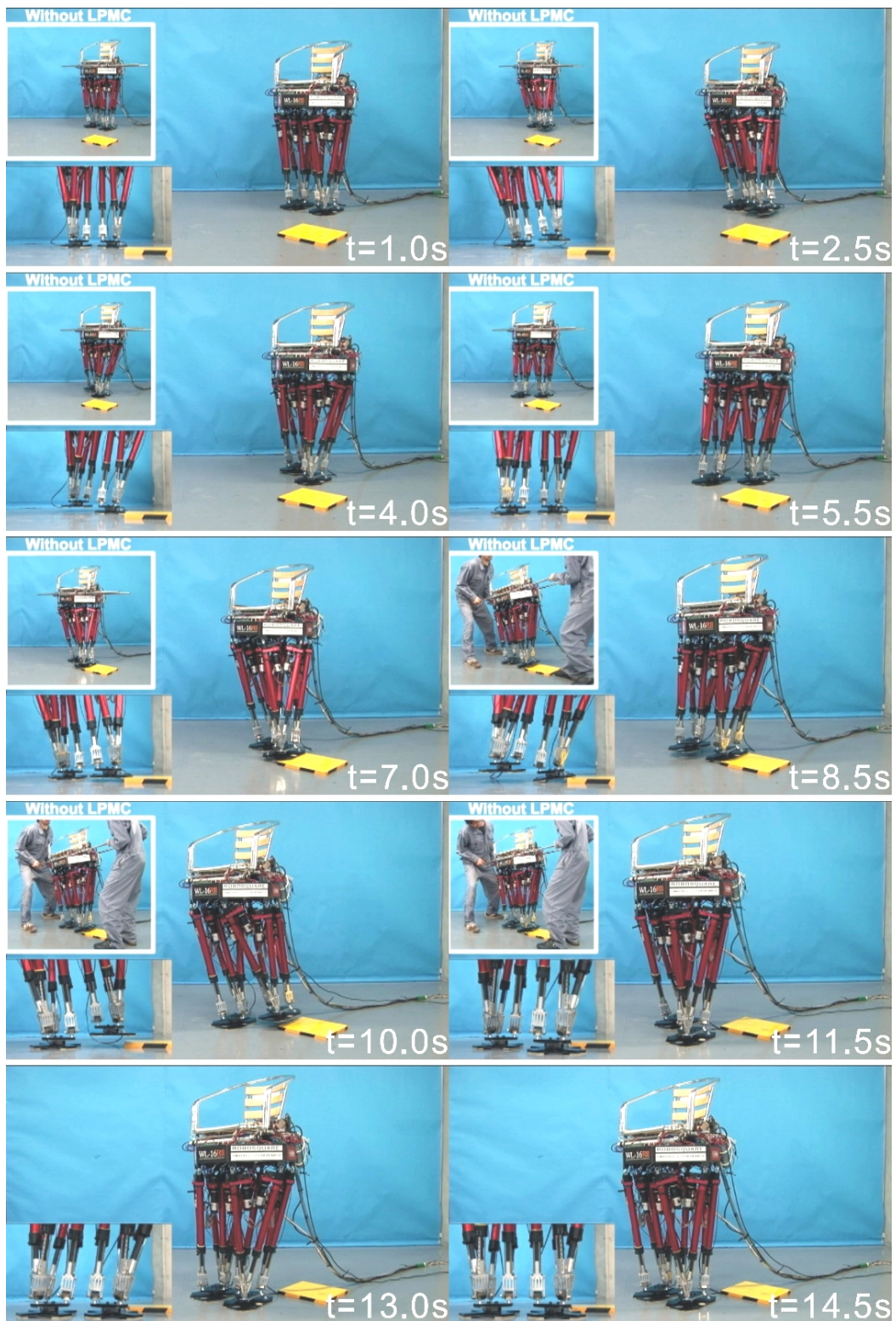
Figure 3.15 Walking experiment, stepping on 20 mm board about the roll axis. (Walking forward, walking cycle: 2.0 s/step, step length: 200 mm/step, height of unevenness: 20 mm)
