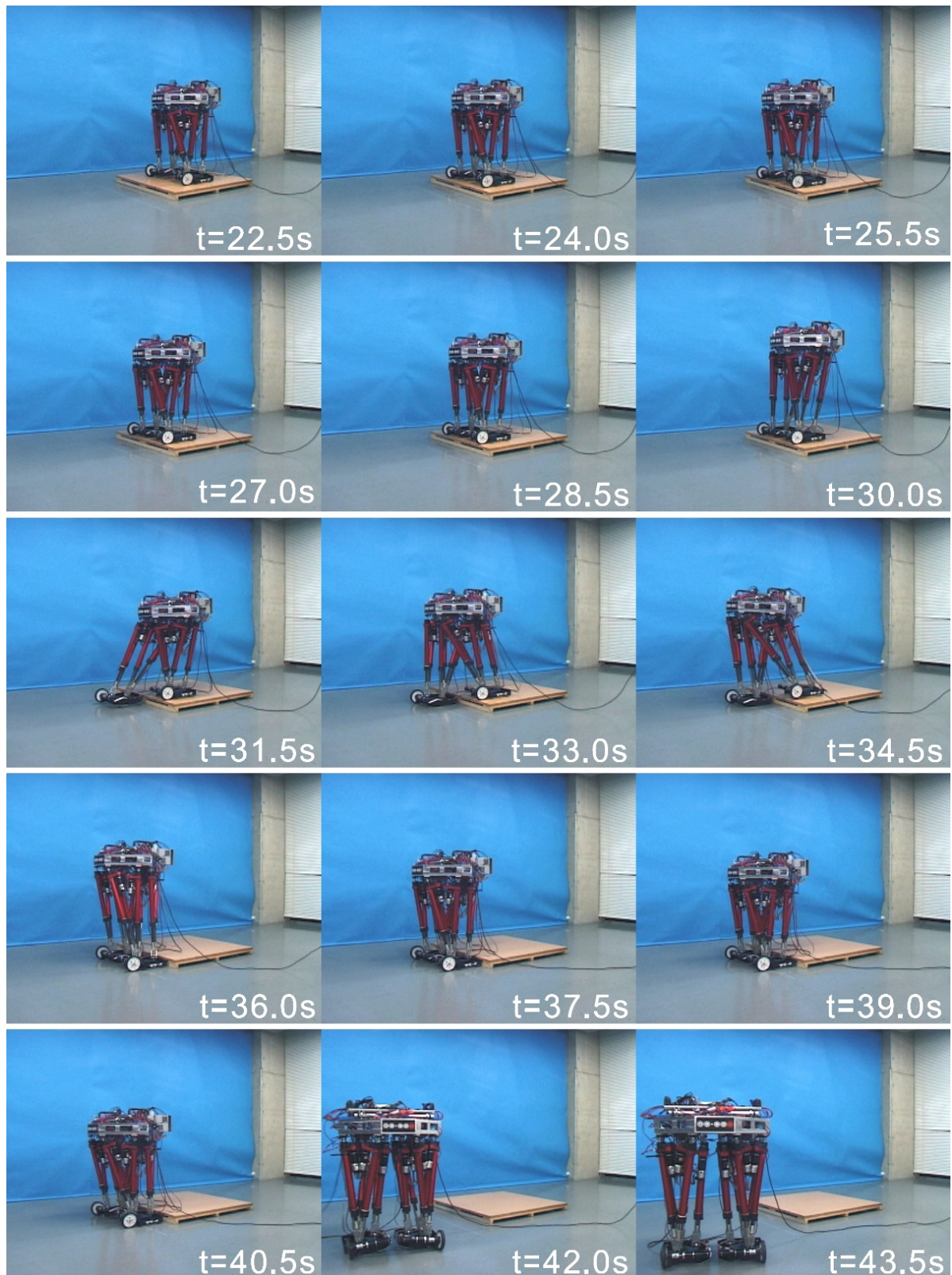
Figure 5.19 Switching between biped walking and wheeled locomotion (2/2).
