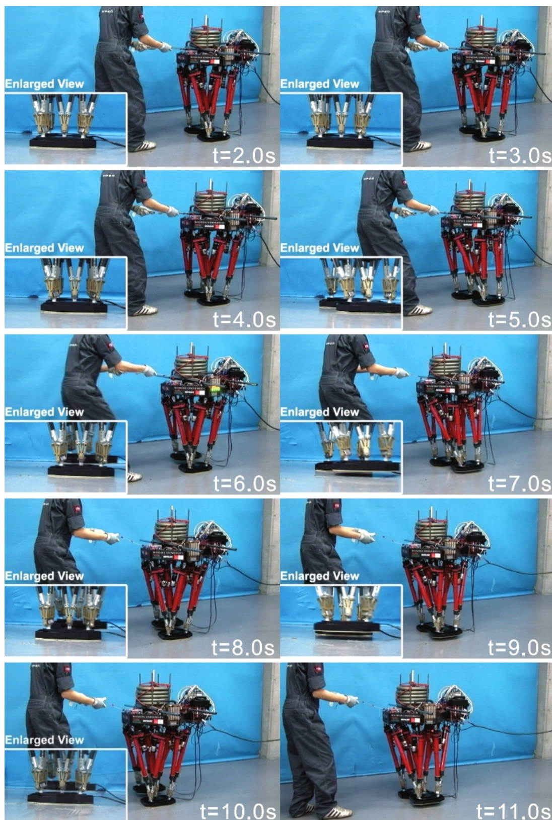
Figure B.34 Walking experiment, pulling the robot forward at the third step. (Walking forward, walking cycle: 1.0 s/step, step length: 100 mm/step, load: 50 kg)
