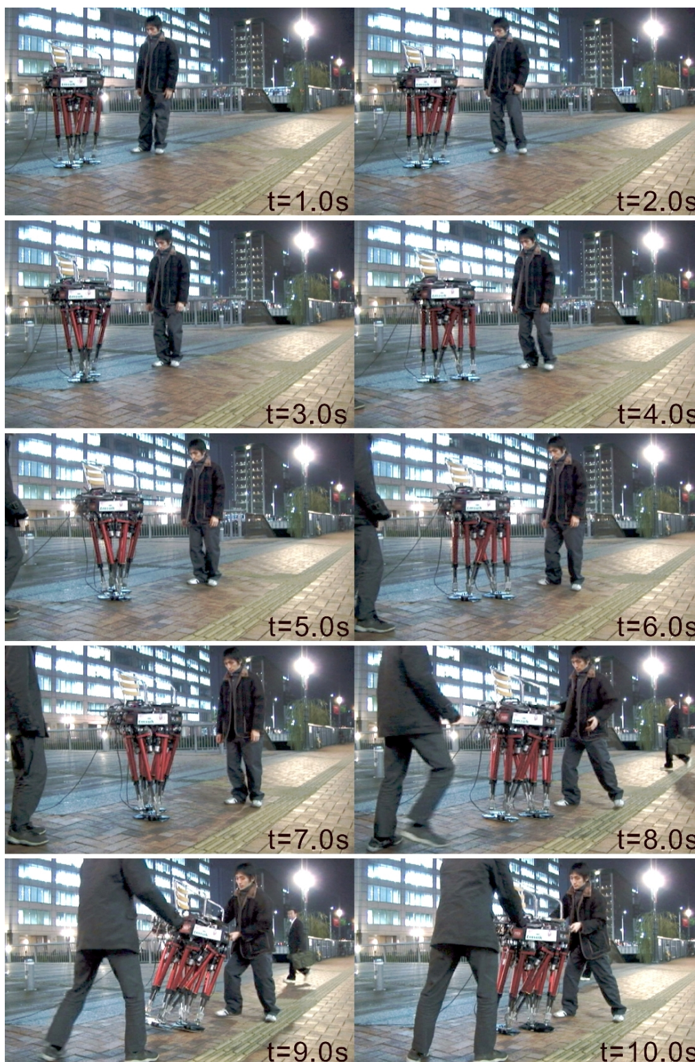
Figure 3.30 Walking experiment on public road in the Fukuoka Special Zones for Robot Development and Test.
