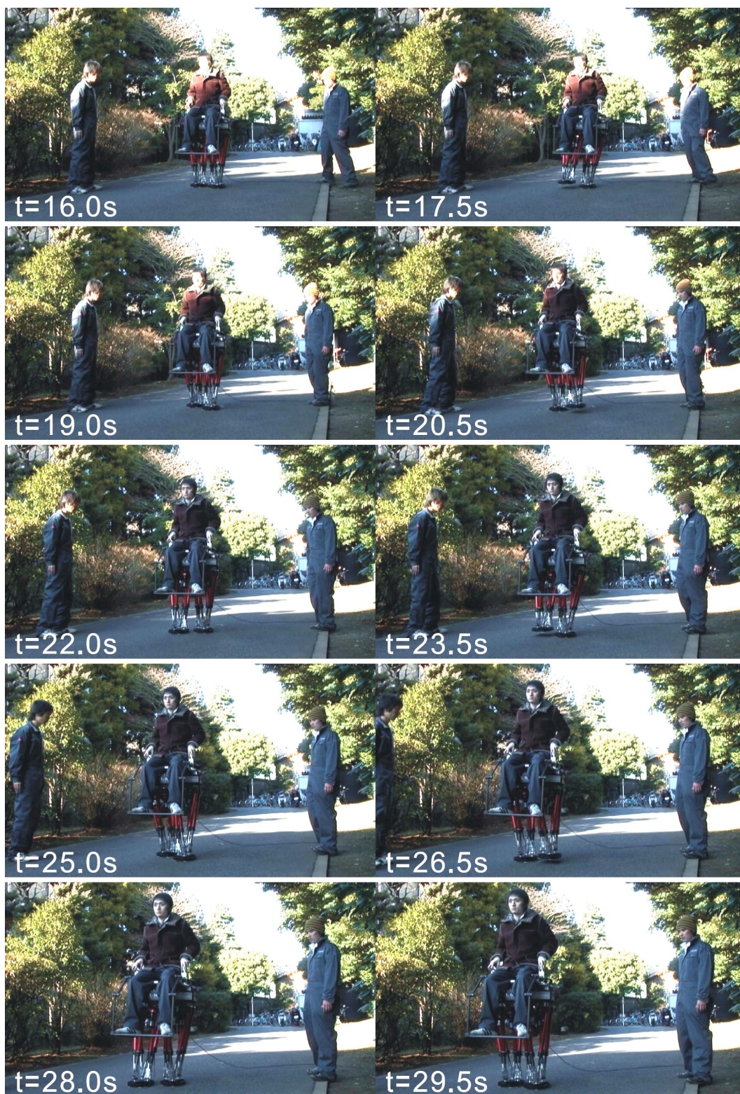
Figure A.35 Walking experiment on the blacktop road, carrying a human (2/2). (Walking forward, walking cycle: 1.0 s/step, step length: 200 mm/step, inclination: 1-2 deg, load: a 55 kg human)
