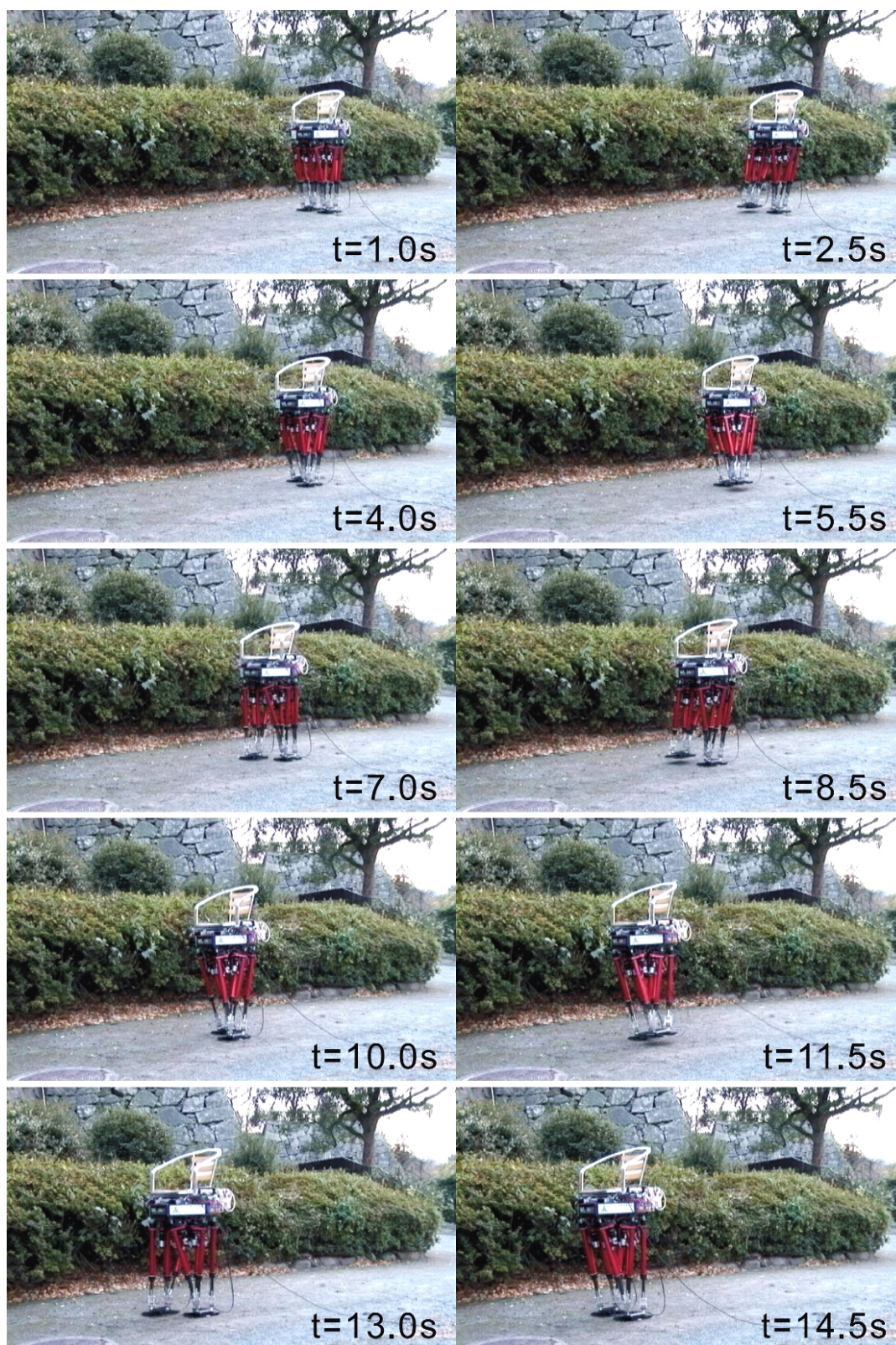
Figure A.14 Walking experiment on gravel road in Fukuoka-kyo castle. (Walking forward, walking cycle: 1.0 s/step, step length: 200 mm/step, inclination: 3 deg)
