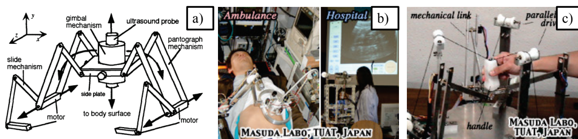
Fig. 1.8 a) Masuda's parallel link slave robot , b) tele-operation examination in the ambulance, c) cable driven haptic device.
