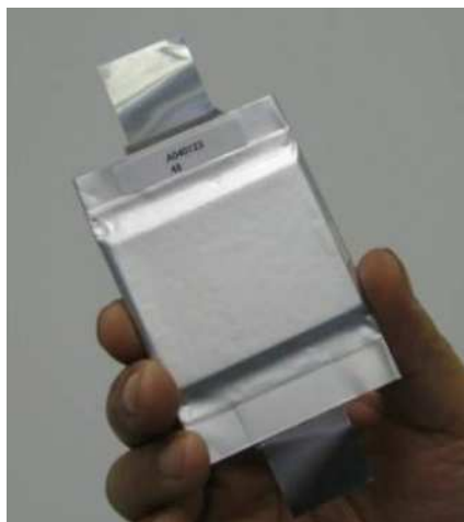
Figure 7.2. An appearance of Al-laminated film packaged organic radical battery.
